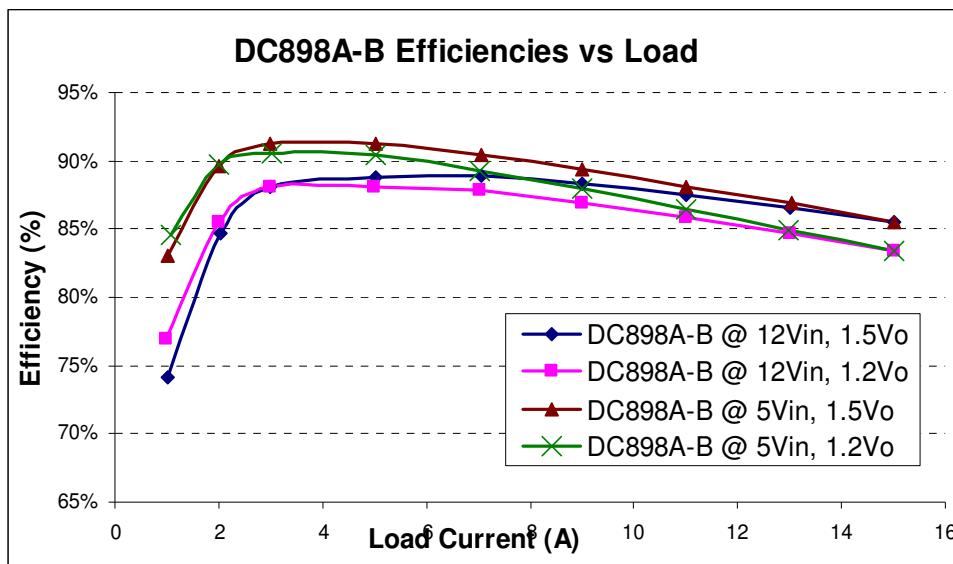
Figure 4. Typical Supply Efficiency vs Load Current of DC898A-B
