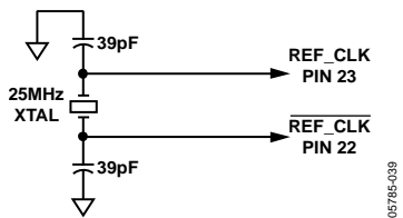
Figure 40. Crystal Configuration for Reference Clock Source
