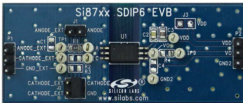
Figure 3. Si871x SDIP6 Evaluation Board Overview
