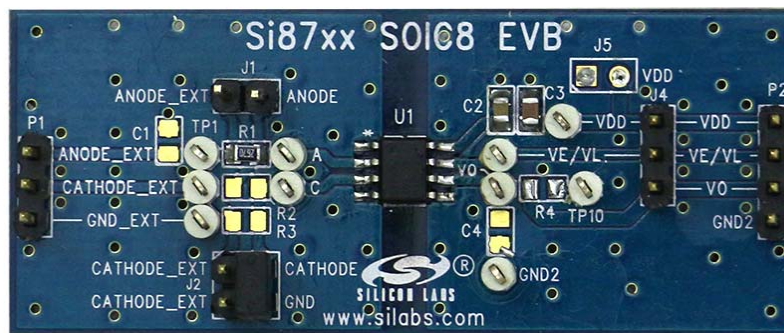
Figure 2. Si871x SOIC8 Evaluation Board Overview
