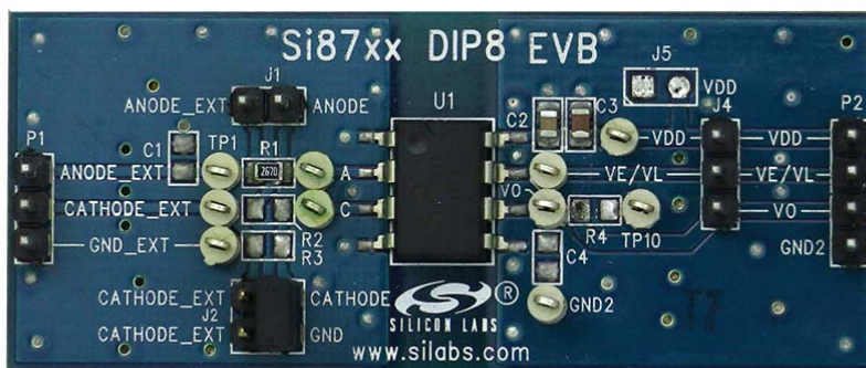
Figure 1. Si871x DIP8 Evaluation Board Overview
