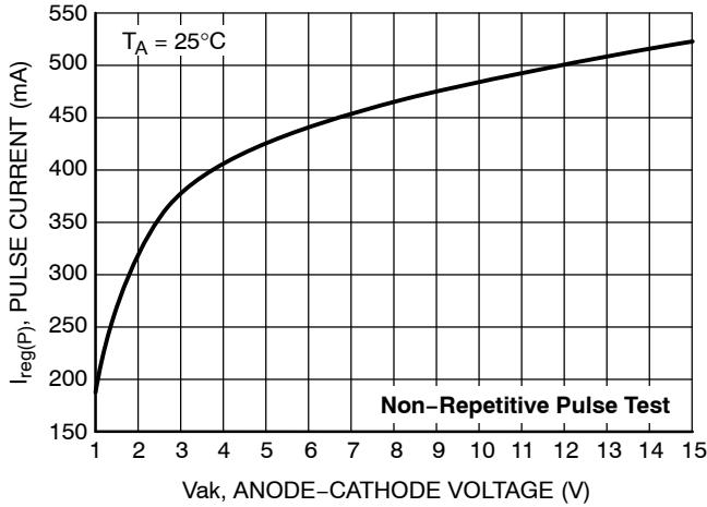
**Figure 3. Pulse Current (I<sub>reg(P)</sub>) vs. Anode-Cathode Voltage (Vak)**
