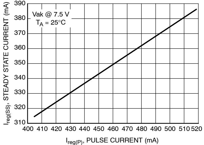
**Figure 4. Steady State Current vs. Pulse Current Testing**
