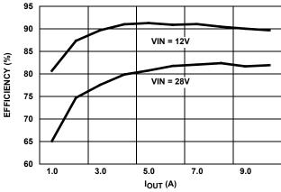
FIGURE 5. EVALUATION BOARD EFFICIENCY (VOLT = 3.3V)
