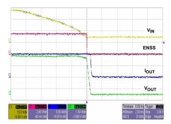
FIGURE 3. POWER-DOWN OF VIN
