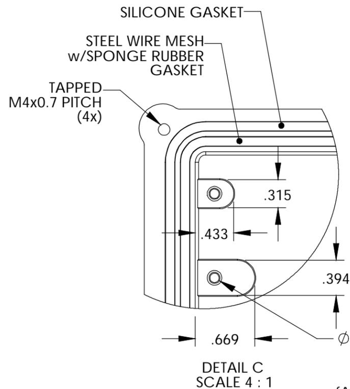
FOUR (4) M4x0.7 PITCH x 20mm (.787") LG. STAINLESS STEEL CAPTIVE SCREWS
