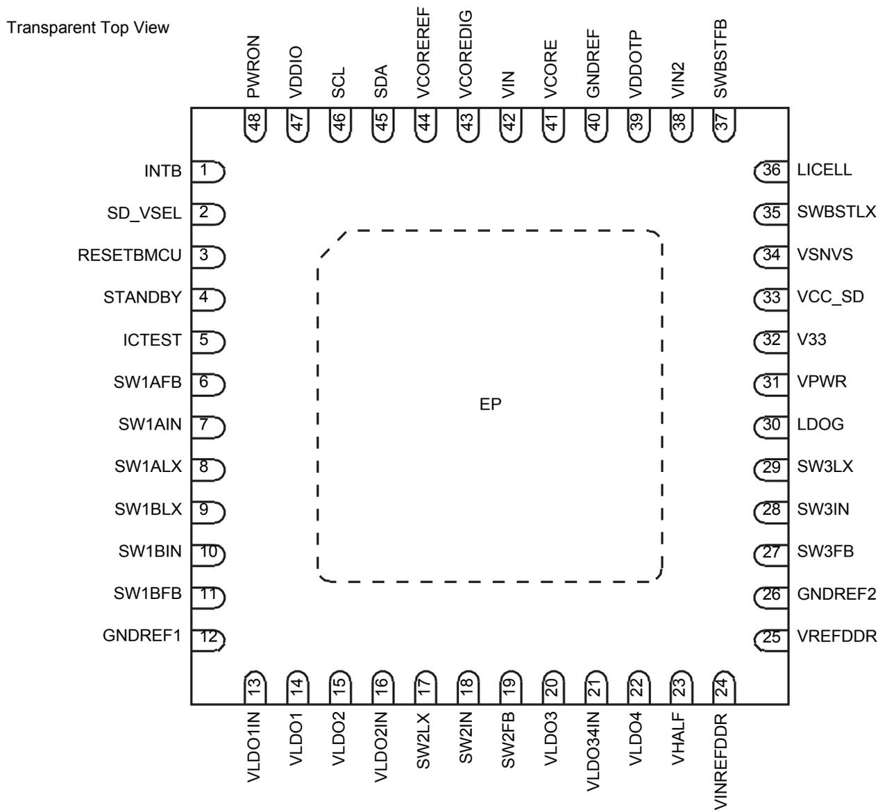
Figure 4. Pinout diagram
