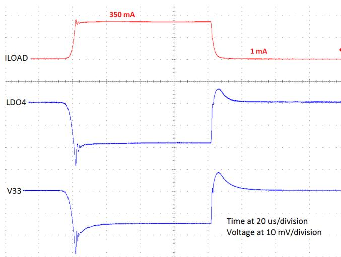
Figure 19. Load transient response - LDO4 and V33
