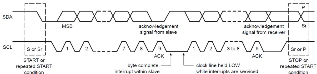
Figure 34. Data transfer on the I<sup>2</sup>C bus
