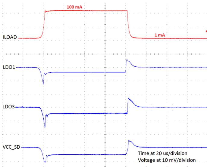
Figure 17. Load transient response - LDO1, LDO3 and VCC\_SD
