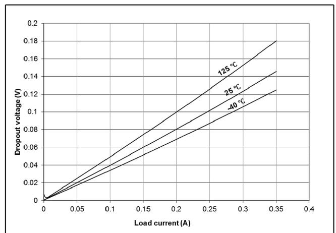
Figure 33. Dropout voltage - VLDO4 -  $V_{OUT} = 1.8\text{ V}$
