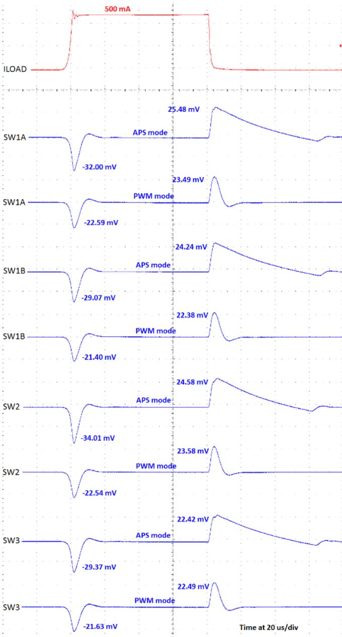
Figure 20. Load transient response - buck regulators
