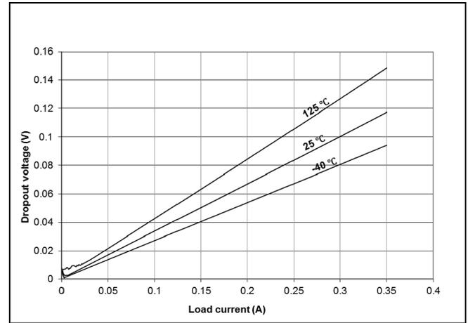
Figure 32. Dropout voltage - VLDO4, V33 -  $V_{OUT} = 3.3\text{ V}$
