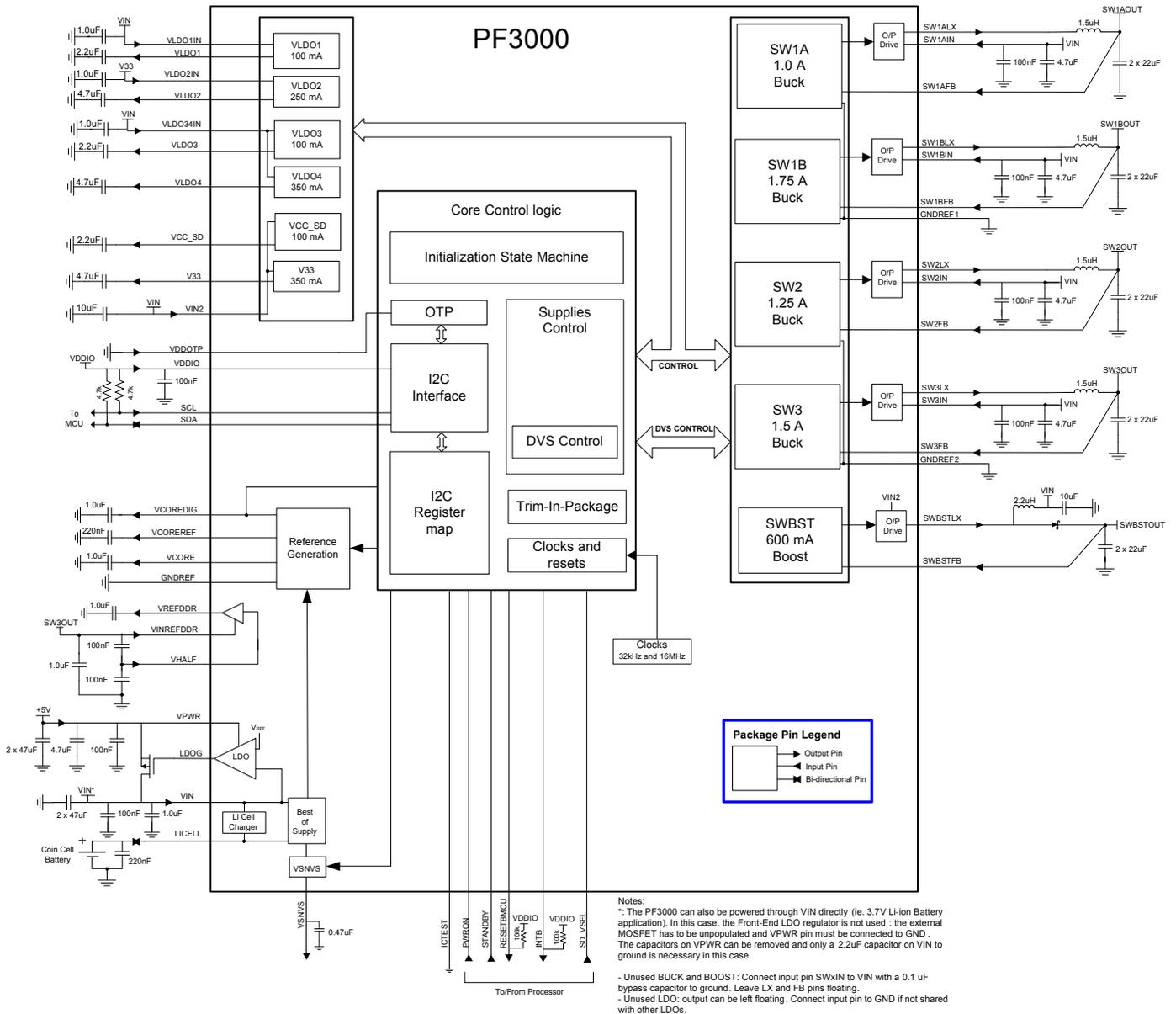
Figure 36. Typical application schematic
