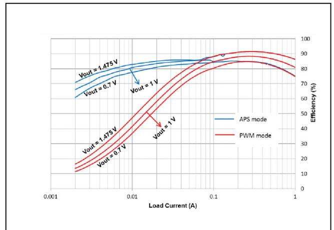
Figure 28. SW1A efficiency - APS and PWM modes
