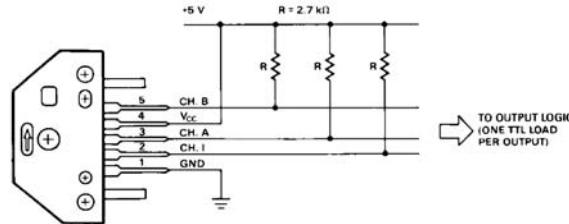
Figure 1. Pull-up Resistors on HEDT-9X40 Encoder Module Outputs.
