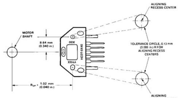
Figure 2. HEDT-9X40 Mounting Tolerance.
