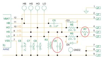
FIGURE 7. RC FILTER ON HS PIN (NOT REQUIRED)
