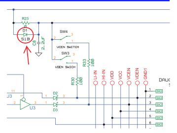
FIGURE 3. DIODE TO SUPPRESS LI-ON BATTERY RIPPLE
