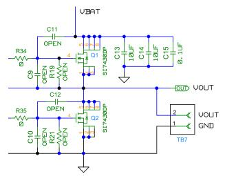
FIGURE 4. OPTIONAL RESISTORS AND CAPACITORS FOR BRIDGE FETS
