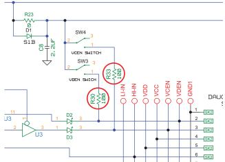
FIGURE 8. VCEN AND VDEN DAMPENING RESISTORS
