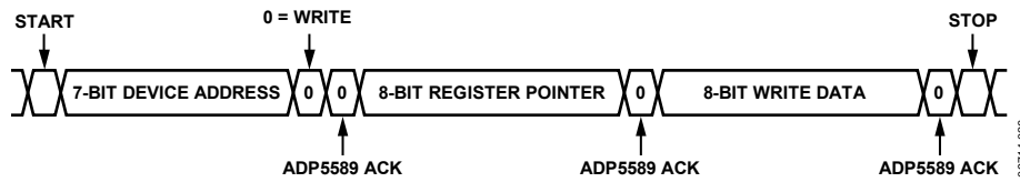
Figure 27. I 2 C Single-Byte Write Sequence
