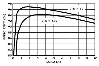
FIGURE 7. EFFICIENCY vs LOAD CURRENT (VOUT = 3.3V)
