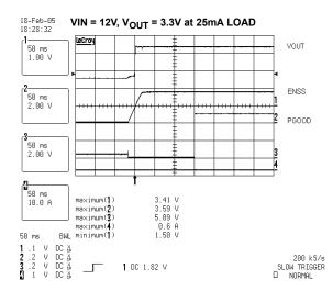
FIGURE 14. PREBIASED OUTPUT AT 25mA LOAD
