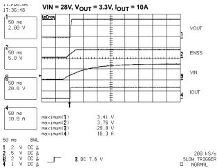
FIGURE 9. TYPICAL SOFT-START WAVEFORM
