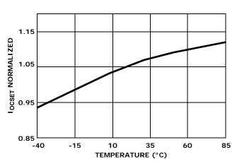
FIGURE 3. IOCSET VS TEMPERATURE
