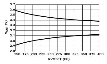
FIGURE 11. VOLTAGE MARGINING vs. VMSET RESISTANCE
