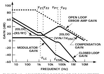
FIGURE 18. ASYMPTOTIC BODE PLOT OF CONVERTER GAIN
