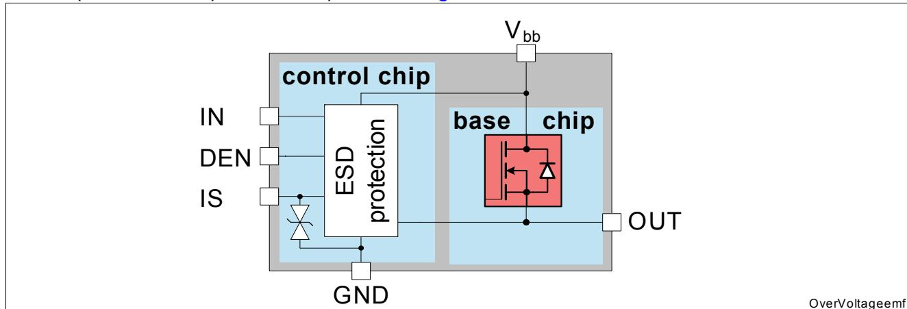
**Figure 18** Over-Voltage Protection
