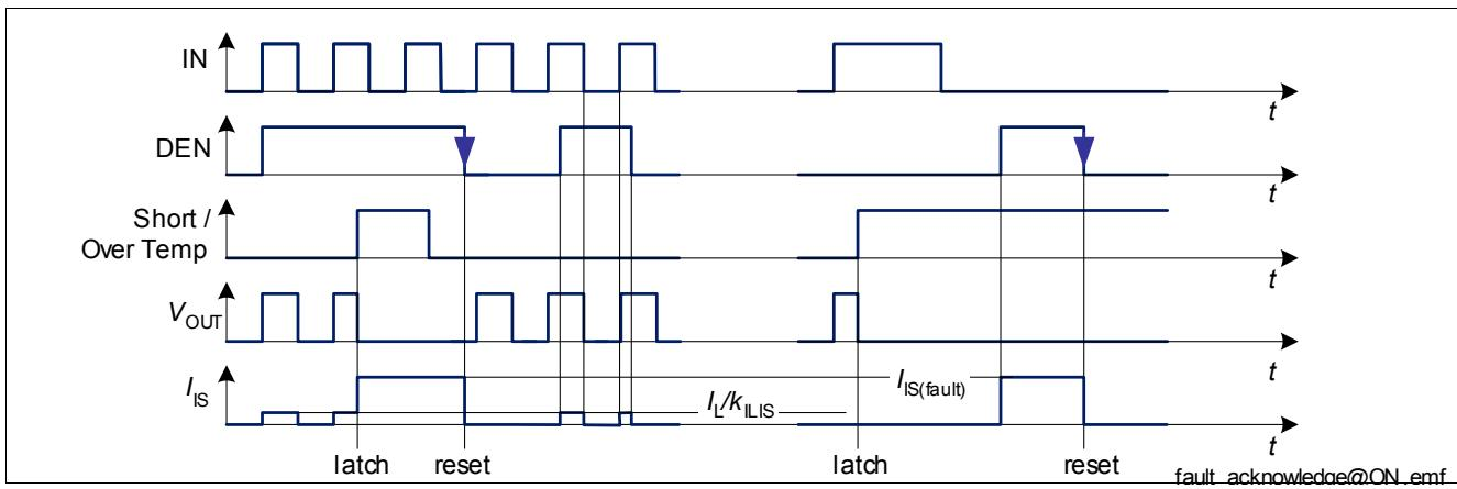
**Figure 24 Fault acknowledge and latch reset**
