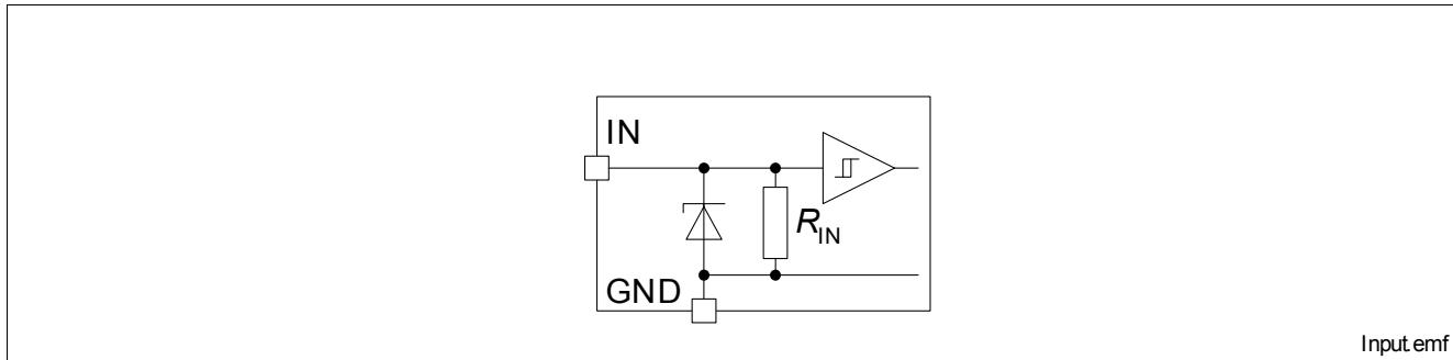
**Figure 5** Input Circuit
