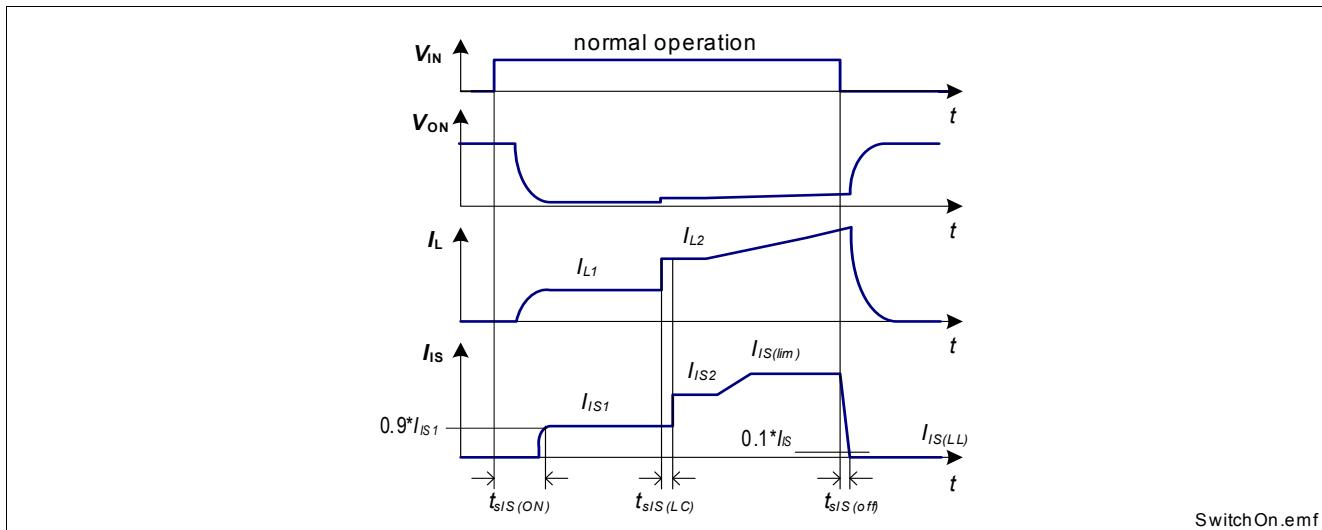
**Figure 21 Timing of Diagnosis Signal in ON-state**
