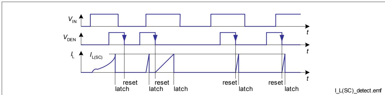
**Figure 14 Shutdown by short circuit current detection**
