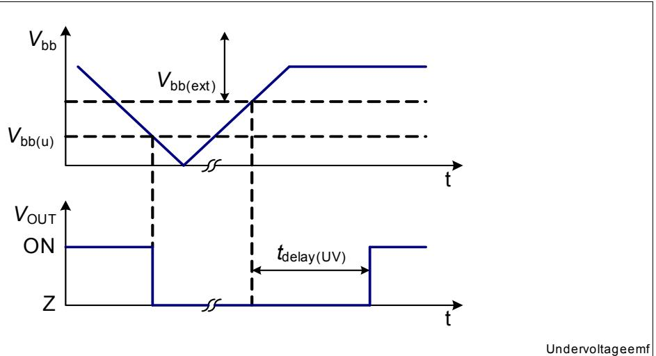
Figure 13 Undervoltage shutdown and restart
