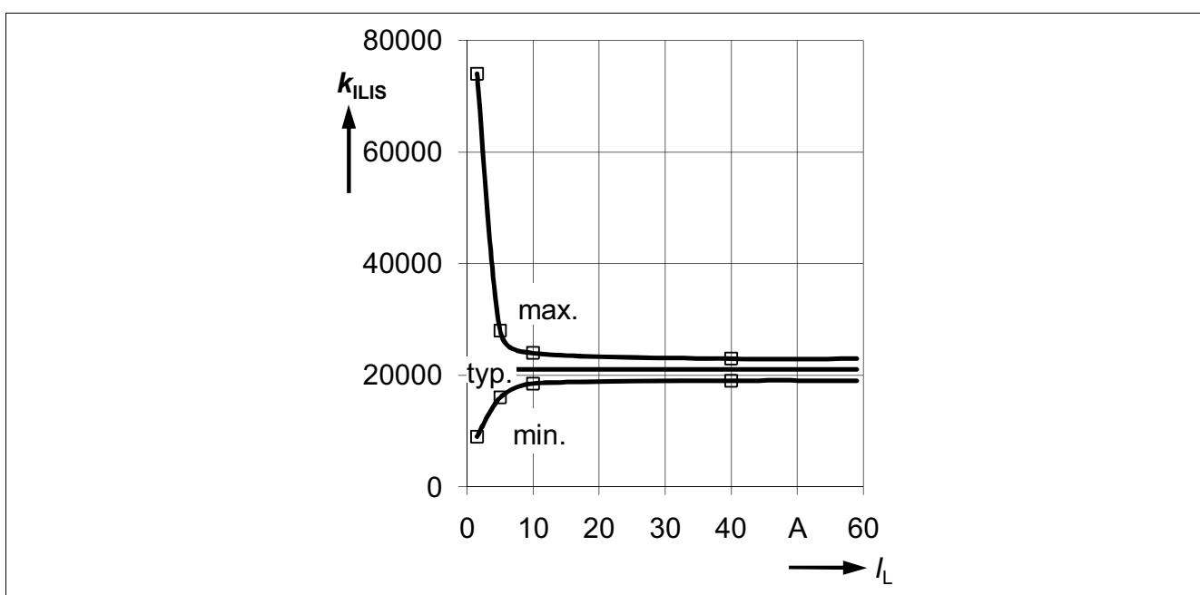
**Figure 22 Current sense ratio  $k_{ILIS}$ <sup>1)</sup>**
