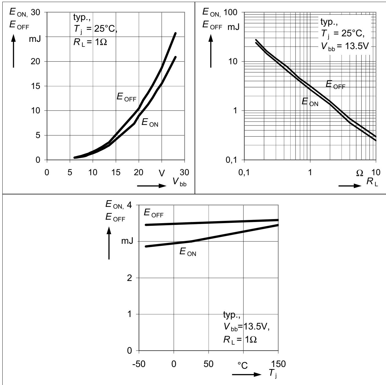
Figure 8 Typical switching losses  $E_{ON}$  and  $E_{OFF}$
