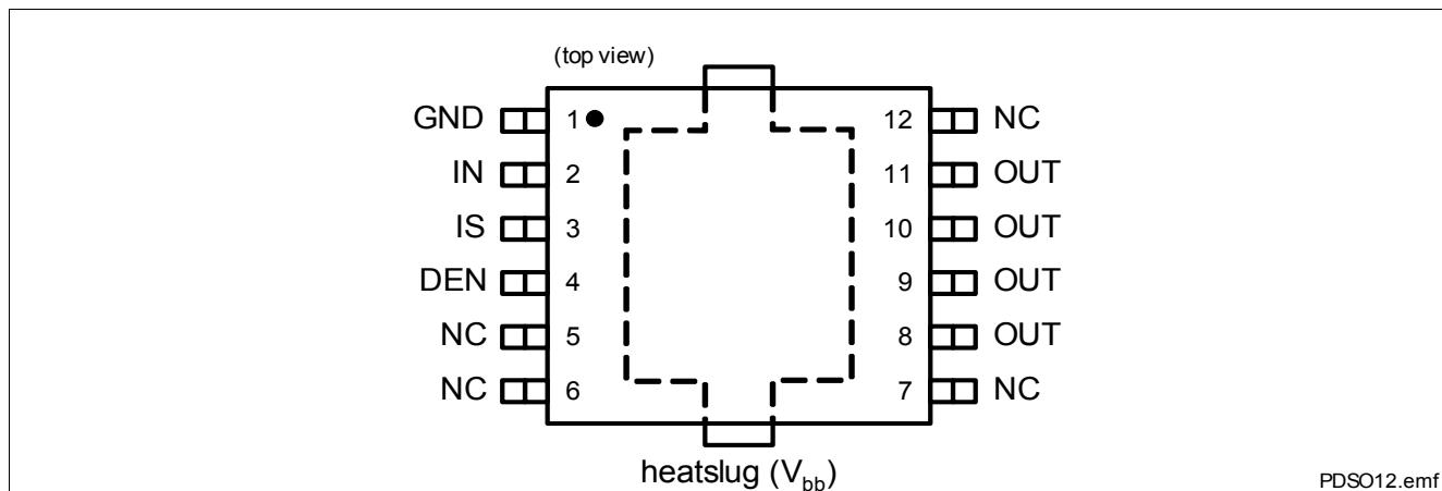
Figure 3 Pin Configuration
