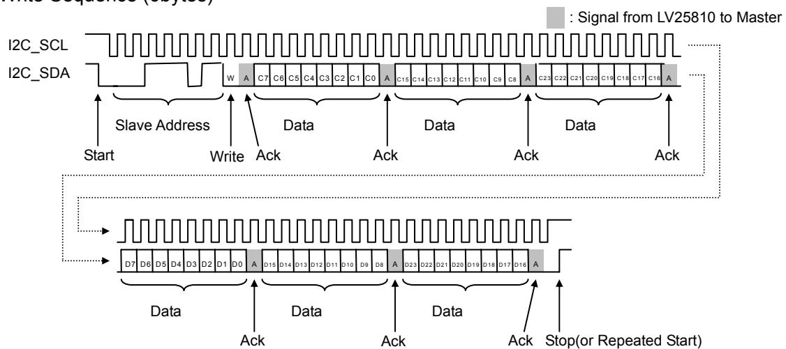
Data write can be accepted during the status of “BUSY” output level is “L”. The command and data during the status of “BUSY” output level is “H” cannot be acceptable.
