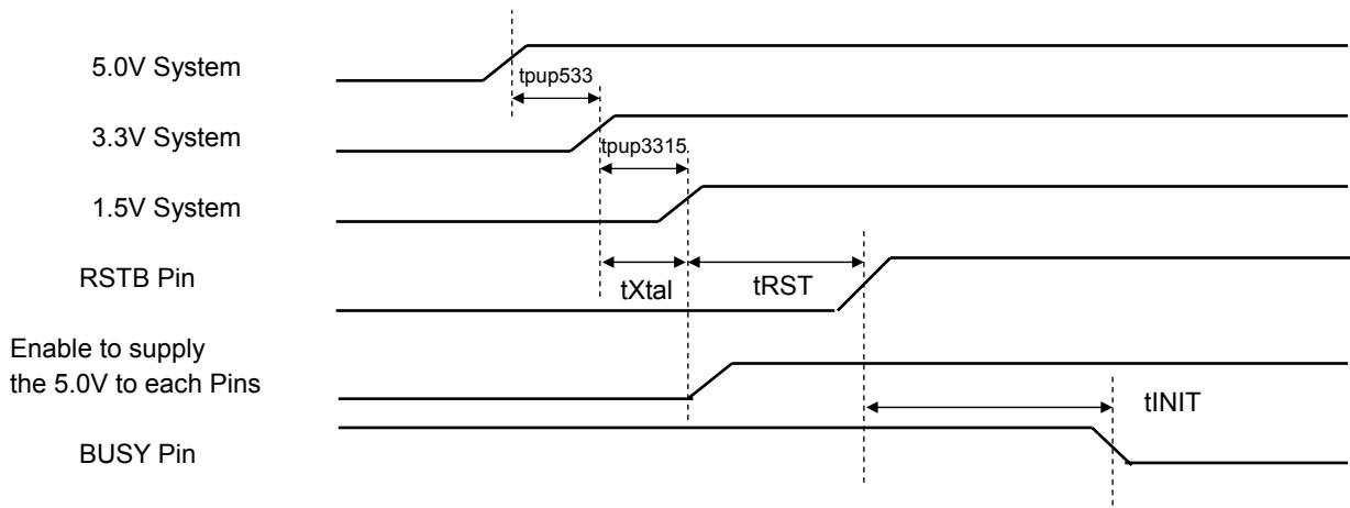
RSTB pin must be kept the “L” level during 5ms after latter either the 1.5V System is activated or the waiting time of the OSC being stable.
