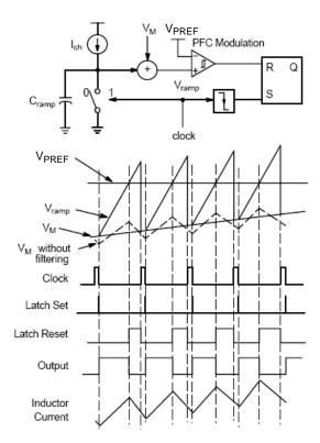
Figure 43. PFC Duty Modulation and Timing Diagram
