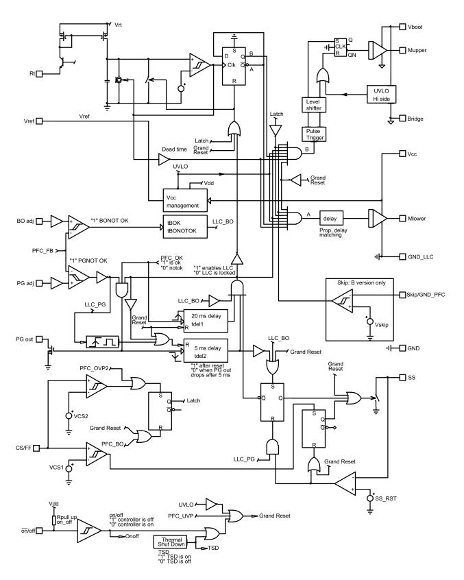
Figure 5. Internal LLC Block Diagram
