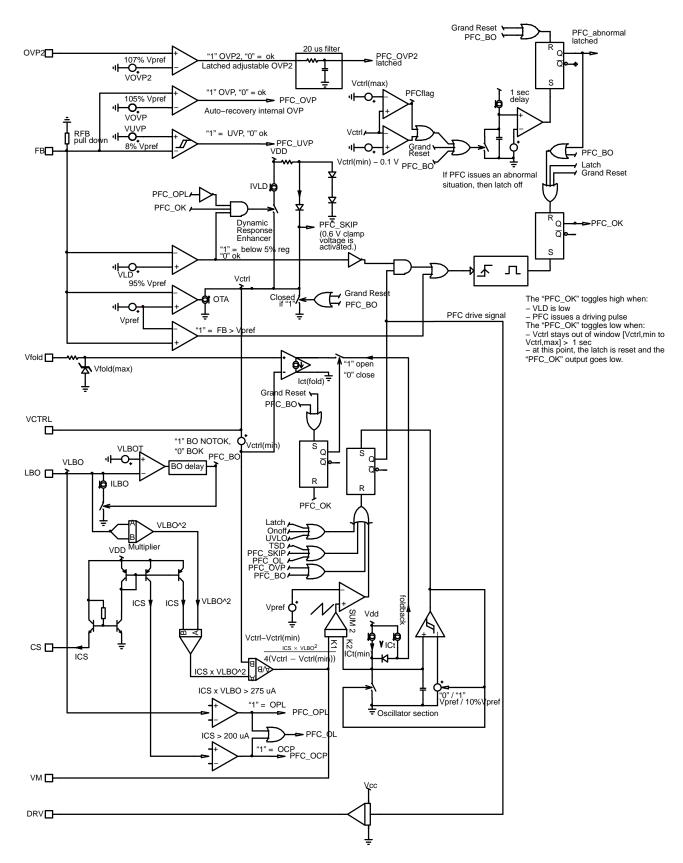
Figure 4. Internal PFC Block Diagram
