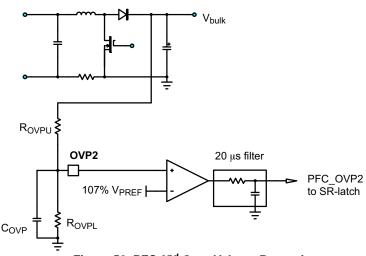
Figure 56. PFC 2<sup>nd</sup> Over-Voltage Protection
