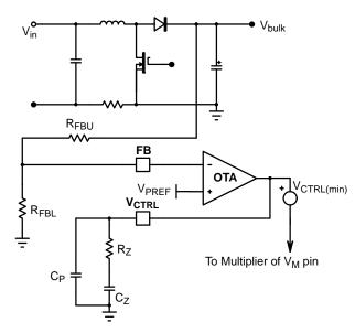
Figure 49. V<sub>CTRL</sub> Type-2 Compensation
