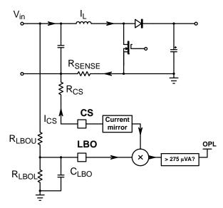
Figure 48. PFC Over-Power Limitation Configuration
