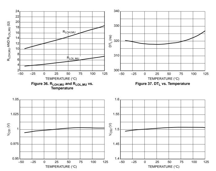
Figure 38. V<sub>CS1</sub> vs. Temperature
