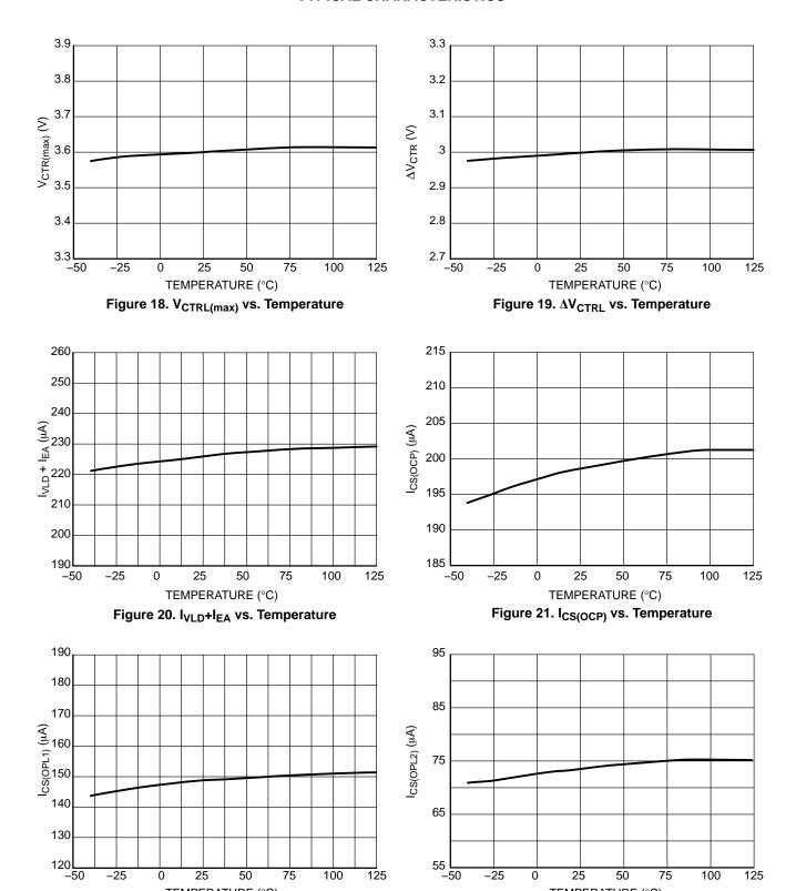
$\label{eq:temperature} \mbox{TEMPERATURE (°C)}$  Figure 22.  $\mbox{I}_{\mbox{CS(OPL1)}}$  vs. Temperature
