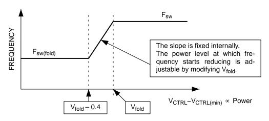
Figure 51. The Relationship between Frequency and V<sub>CTRL</sub>
