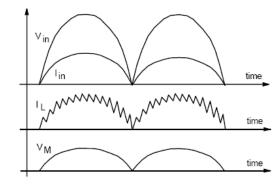
Figure 44. Multiplier Voltage Timing Diagram
