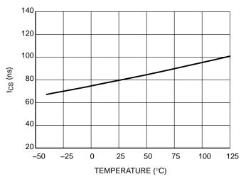
Figure 40.  $t_{\text{CS}}$  vs. Temperature
