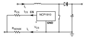
Figure 47. PFC Current Sensing Configuration
