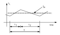
Figure 42. Inductor Current in CCM
