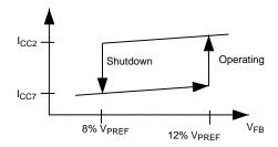
Figure 55. PFC Under-Voltage Protection
