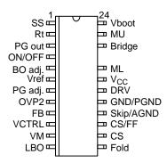
Figure 1. Pin Connections
