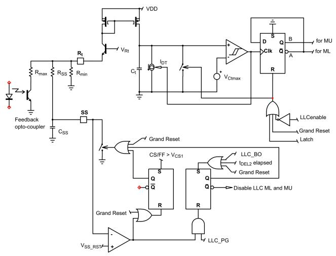
Figure 57. The Current Controlled Oscillator Architecture and Configuration
