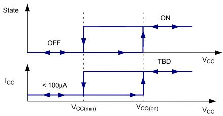
Figure 63. V<sub>CC</sub> Under-Voltage LockOut (UVLO)
