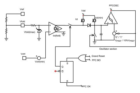
Figure 50. The PFC Frequency Foldback Block
