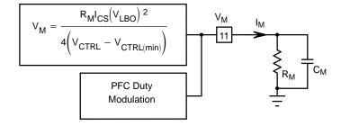
Figure 45. The Multiplier Voltage Pin Configuration
