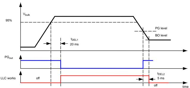
Figure 61. The Timing for t<sub>DEL1</sub> and t<sub>DEL2</sub>
