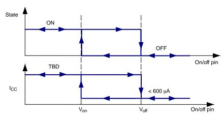
Figure 62. Remote on/off (on/off Pin)
