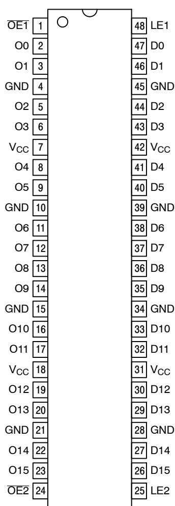
**Figure 1. Pinout: 48-Lead
