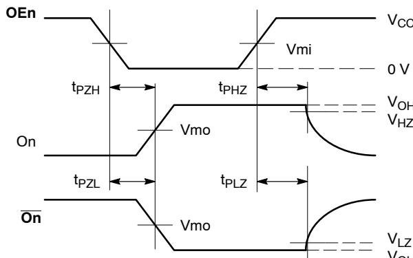
**WAVEFORM 2 – OUTPUT ENABLE AND DISABLE TIMES**
