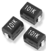
Specially developed for automatic mounting applications, this exciting range of chip inductors are ferrite based and sealed in a thermoset plastic body. They employ solder coated copper terminations with barrier layer. Customers can therefore expect consistent quality, performance and reliability. Its smooth top surface makes it particularly well suited to pick and place equipments.
