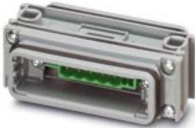
D-SUB coupling, for DeviceNet, shell size 3, header, unshielded, connection direction straight, IP67 degree of protection
