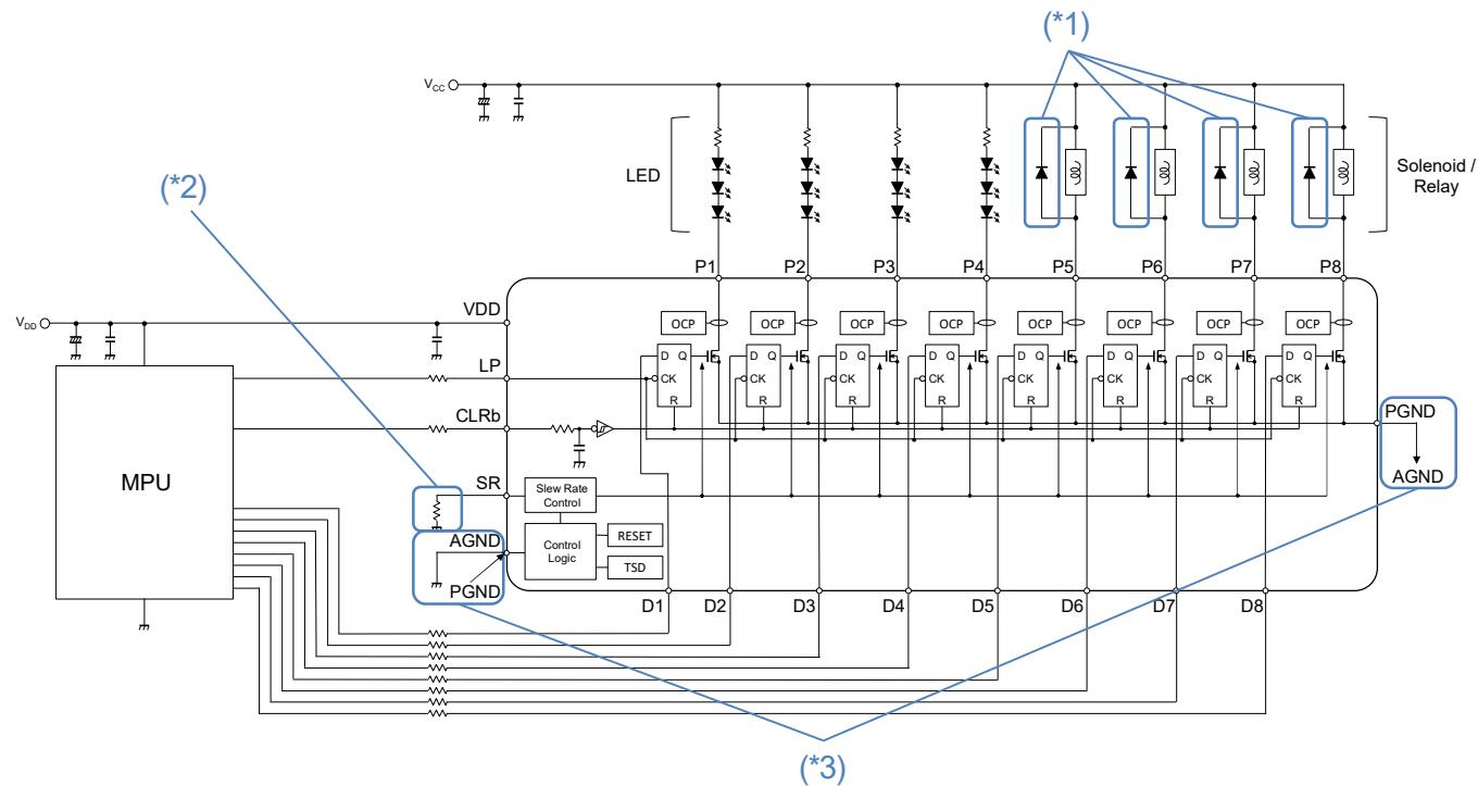
(\*1): The output pins don't have clamp circuits.
