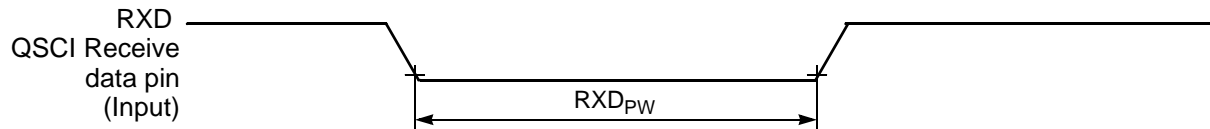
Figure 10-12 RXD Pulse Width
