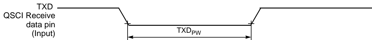
Figure 10-13 TXD Pulse Width
