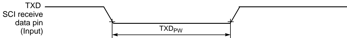
Figure 3-26 TXD Pulse Width
