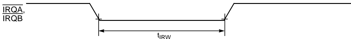
Figure 3-13 External Interrupt Timing (Negative-Edge-Sensitive)
