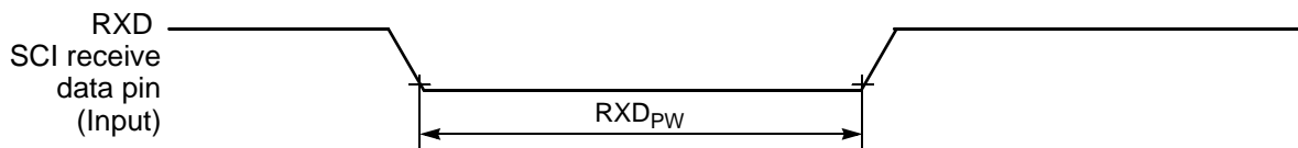
Figure 3-25 RXD Pulse Width
