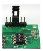
Set the Mode Switch to Mode1 (as above) and place a jumper between Pin3 and Pin4 of the PICkit programming connector (as shown in the picture) before power up or reset.
