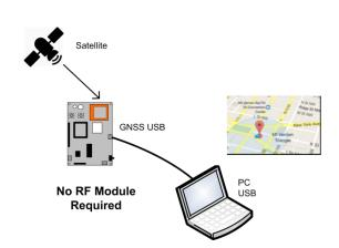
This mode allows the GNSS module serial data to be directly accessed by connecting a cable between the board GNSS micro USB connector (note position) and a PC USB port.
