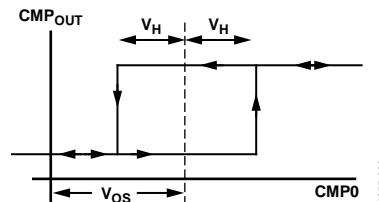
Figure 56. Comparator Hysteresis Transfer Function
