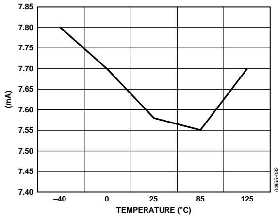
Figure 31. Current Consumption vs. Temperature @ CD = 7
