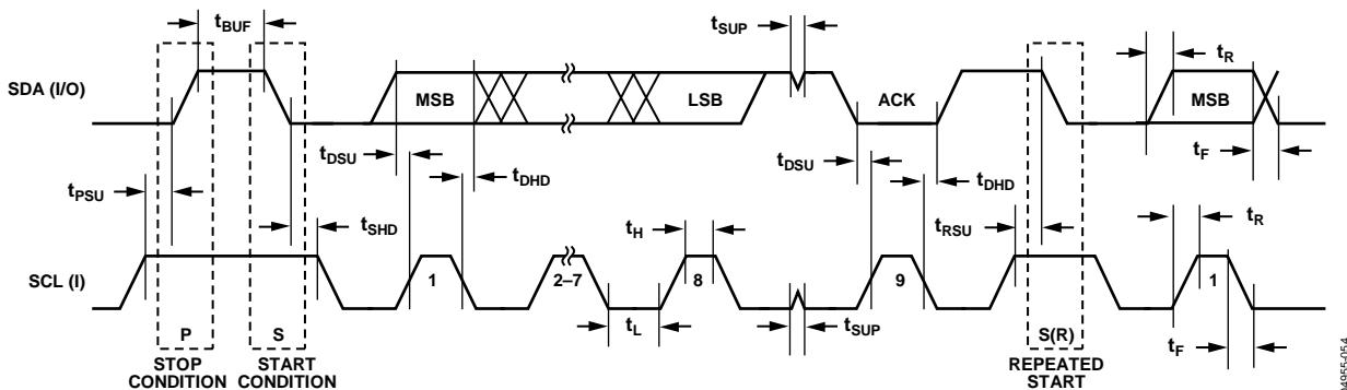
Figure 5. I<sup>2</sup>C Compatible Interface Timing
