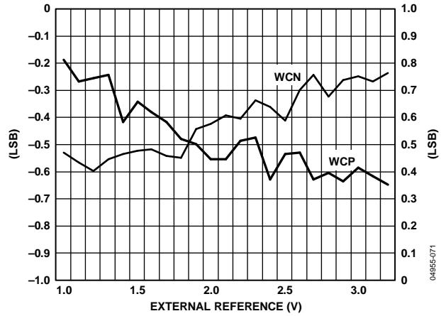
Figure 23. Typical Worst-Case (Positive (WCP) and Negative (WCN)) DNL Error vs.  $V_{REF}$ ,  $f_s = 774\text{ kSPS}$
