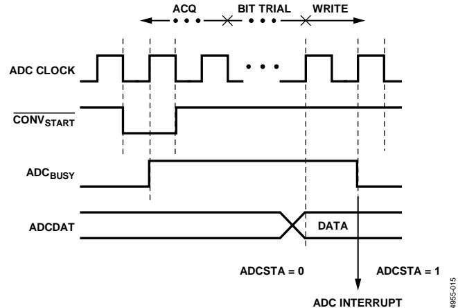
Figure 42. ADC Timing
