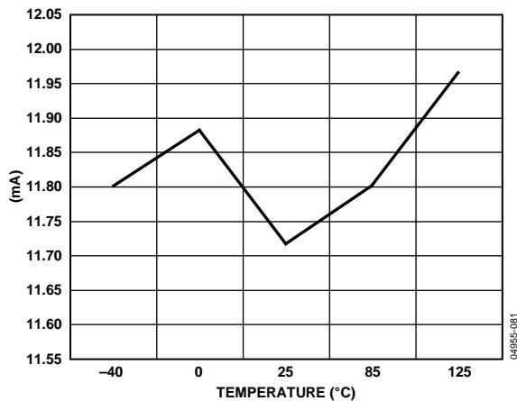
Figure 30. Current Consumption vs. Temperature @ CD = 3
