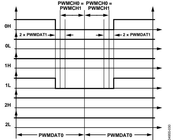
Figure 61. Active Low PWM Signals Suitable for ECM Control,
