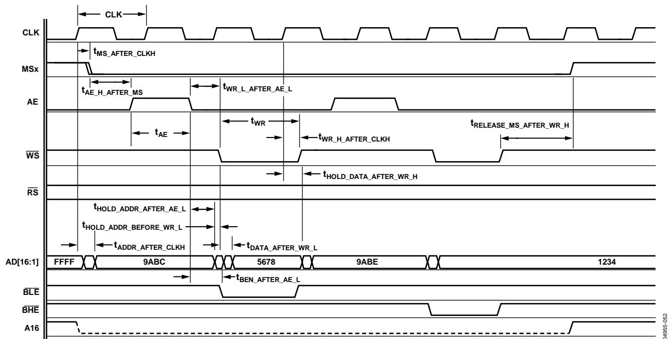
Figure 3. External Memory Write Cycle (See Table 78)
