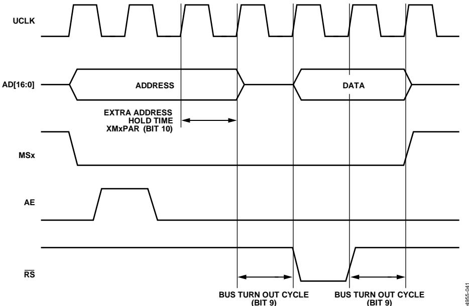
Figure 72. External Memory Read Cycle with Address Hold and Bus Turn Cycles
