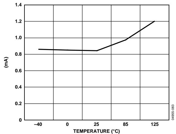
Figure 32. Current Consumption vs. Temperature in Sleep Mode
