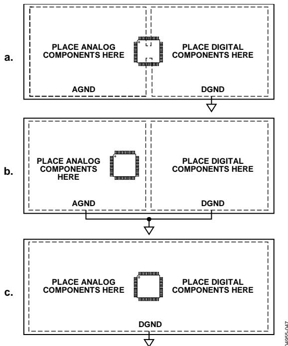
Figure 79. System Grounding Schemes
