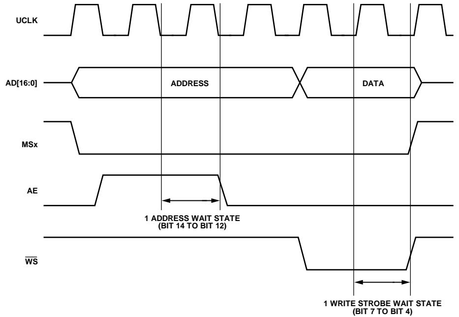
Figure 74. External Memory Write Cycle with Wait States
