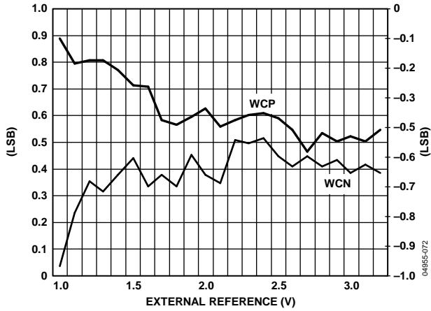
Figure 20. Typical Worst-Case (Positive (WCP) and Negative (WCN)) INL Error vs.  $V_{REF}$ ,  $f_s = 774\text{ kSPS}$
