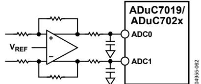
Figure 50. Buffering Differential Inputs
