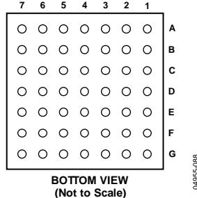
Figure 17. 49-Ball BGA Pin Configuration (ADuC7029)
