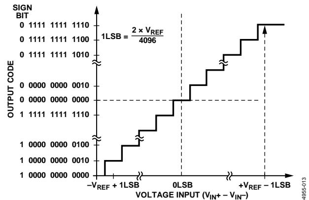
Figure 40. ADC Transfer Function in Differential Mode
