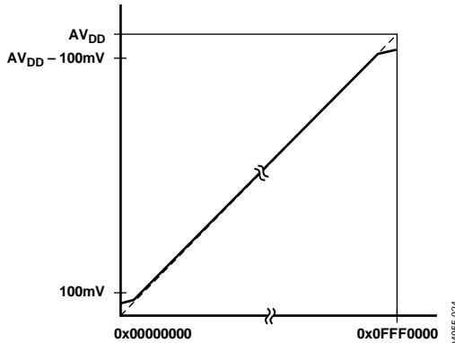
Figure 54. Endpoint Nonlinearities Due to Amplifier Saturation
