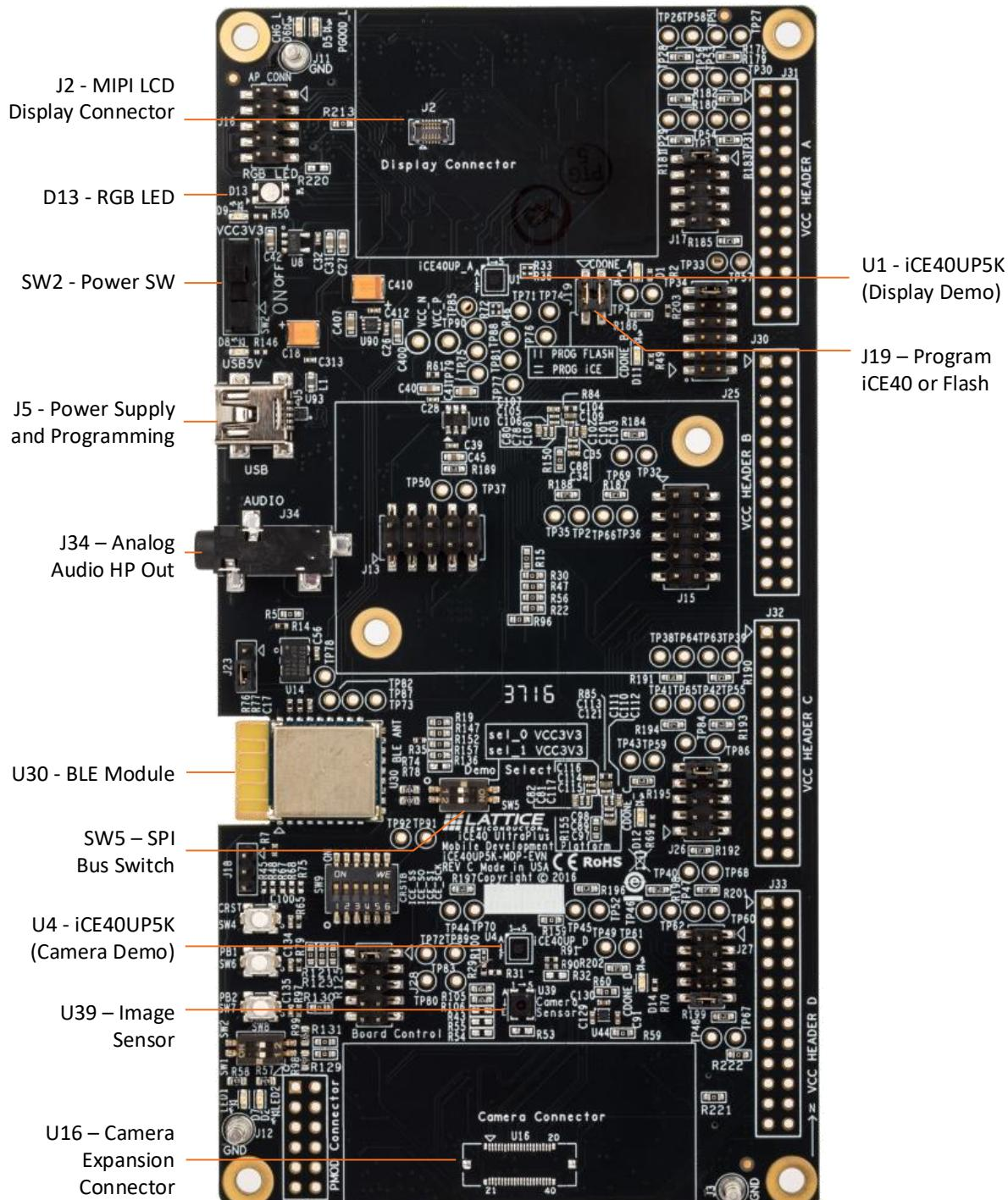
Figure 2.1. iCE40 UltraPlus Mobile Development Platform Board (Top Side)
