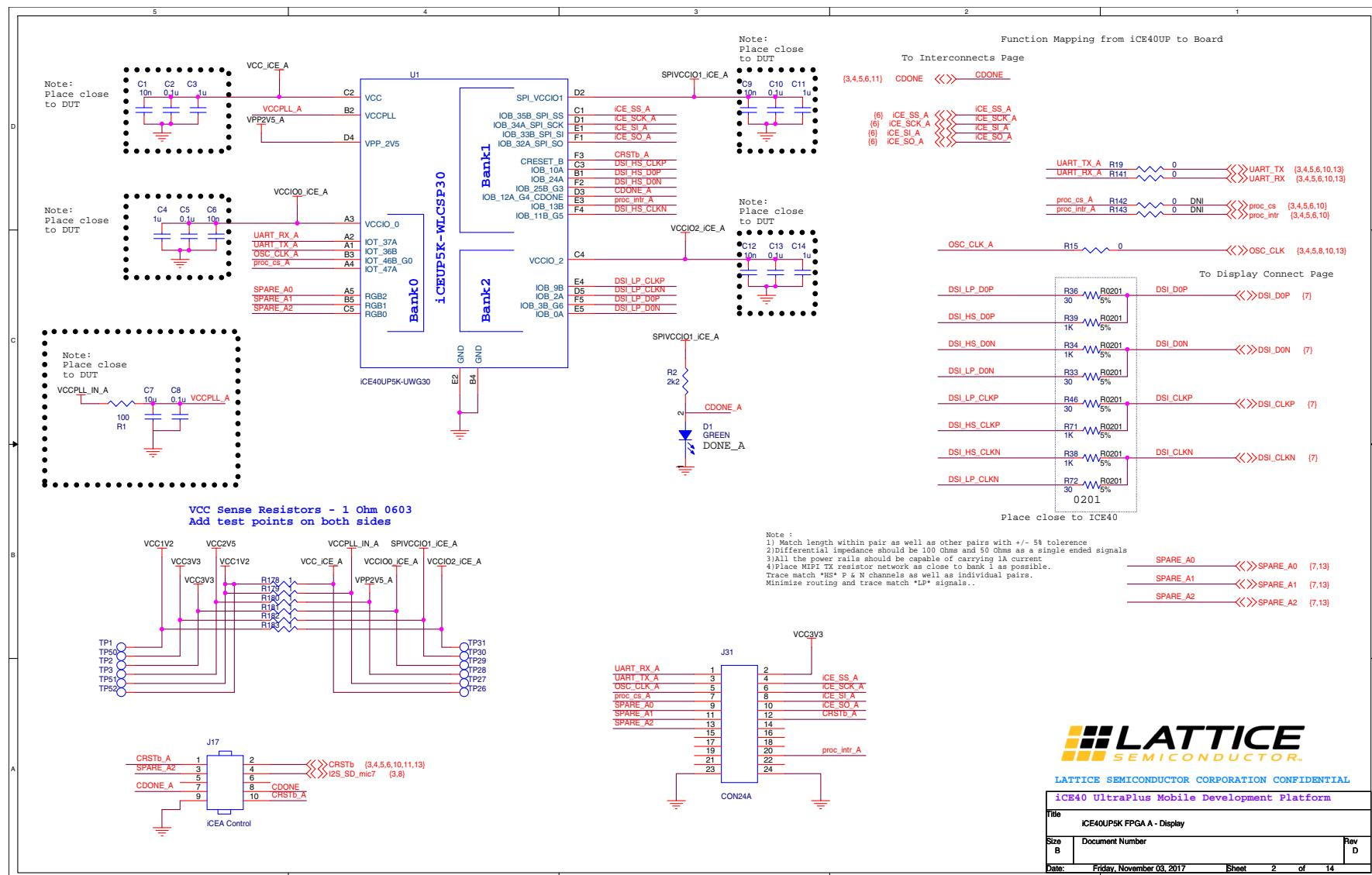
Figure A.2. iCE40UP5K FPGA A - Display
