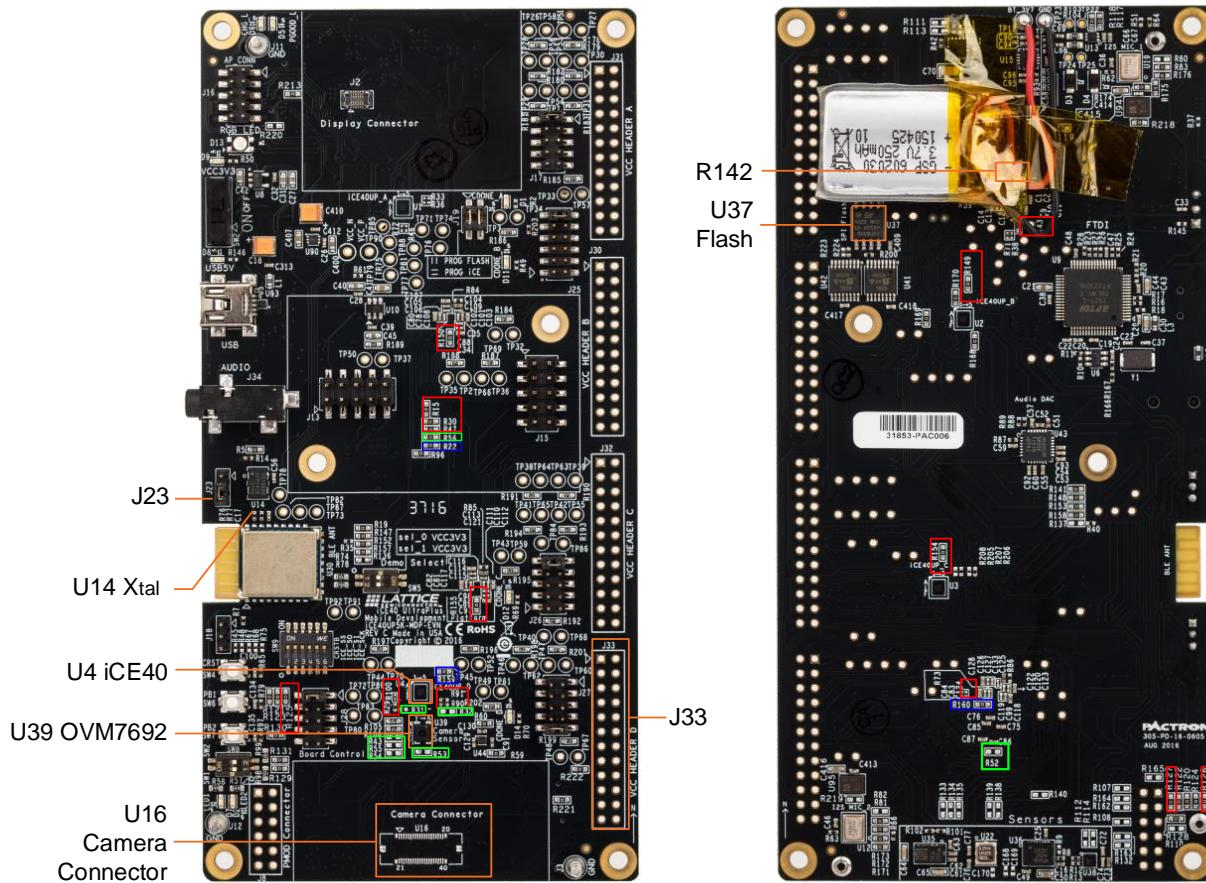
**Figure 6.1. Rework Resistor Positions Described in Parallel Video Bus Configuration**
