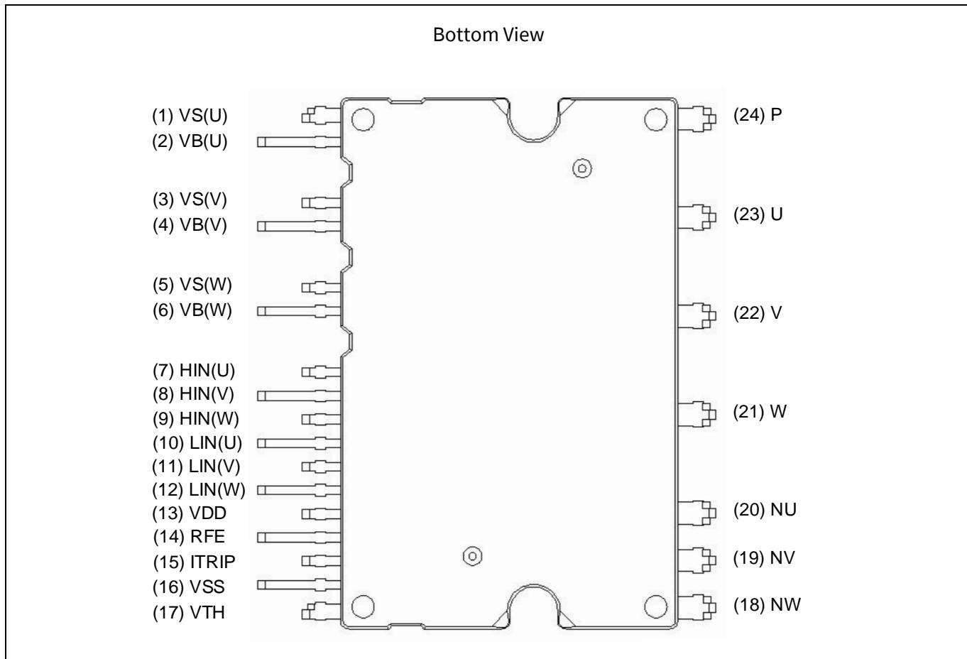
**Figure 2 Module pinout****Table 2 Pin Assignment**
