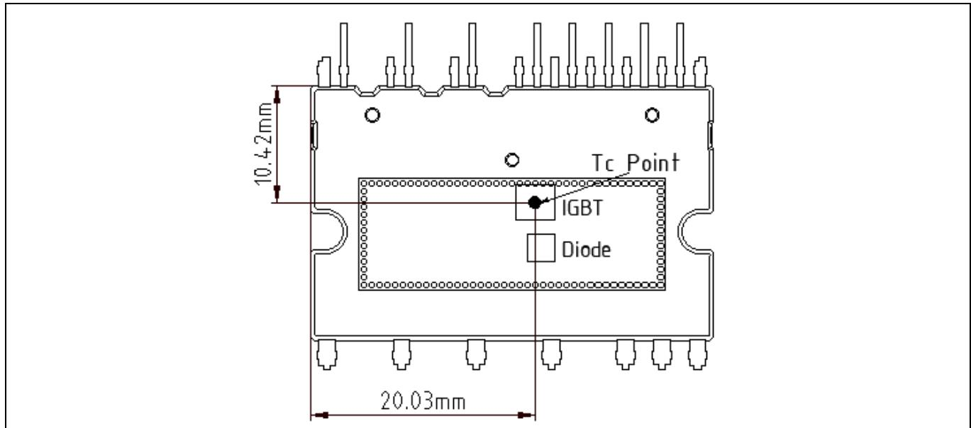
Figure 7  $T_c$  measurement point<sup>1</sup>
