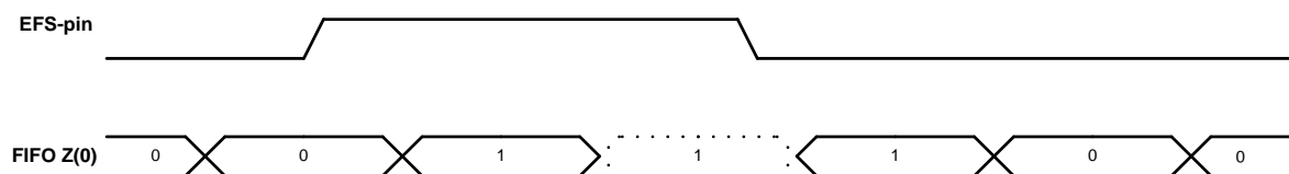
Figure 35: Timing diagram for external FIFO synchronization.
