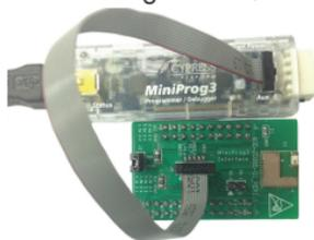
**Fig 3: Programming/Debugging with MiniProg3**
