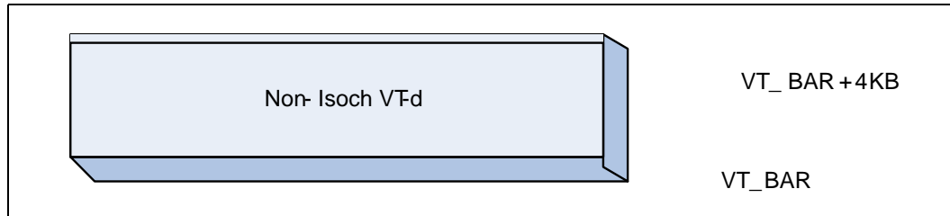
Figure 21-2. Base Address of Intel VT-D Remap Engines
