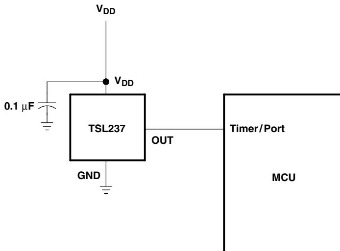
**Figure 9. Typical TSL237 Interface to a Microcontroller**
