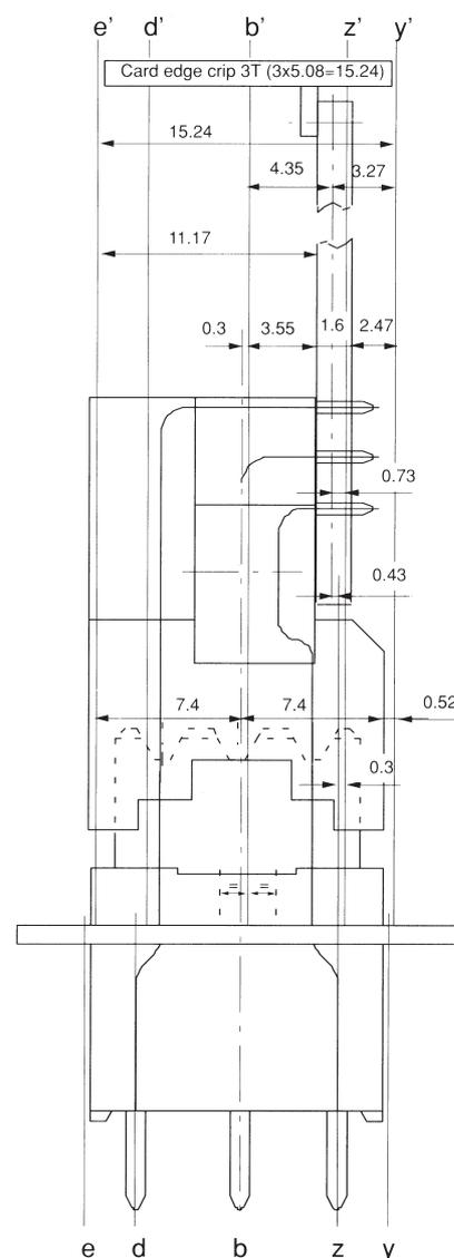
These drawings contain important dimensions for the use of DIN 41612/IEC 60603-2 connectors in 19" rack systems.
