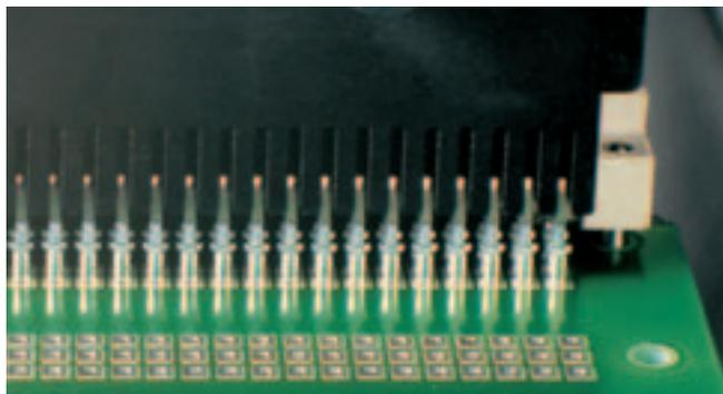
The male connectors and the inverted female connectors have right-angled pressfit terminations with a shoulder. The appropriate press-in tool with matching cavities, enables the pressfitting of the connectors into the PCB. The press-in forces are absorbed by the contact shoulder.
