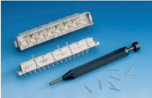
The coding pins are inserted with an insertion tool into predrilled holes located between the contact rows on the female connector. Corresponding holes must then be drilled on the male connector. Recessed hole points on the male connector provides alignment for drilling the corresponding holes.
