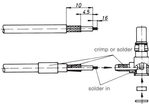
For Straight Coaxial Contact Assembly
