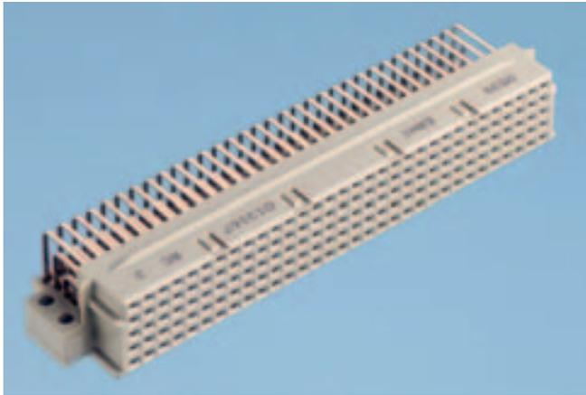
Size TE 160 female connectors are fitted with a locating strip. This plastic component is attached to the extended mounting flanges and serves to guide the pins accurately. The extended mounting flanges have two mounting holes.
