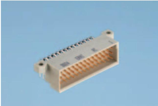
These Eurocard Center connectors fit precisely between two connectors mounted on a standard double Eurocard. The connector mounting flanges are standardized so that the Eurocard Center Connectors can be combined with sizes B, C, D, E, E160, M and H11 male connectors and with the size Q and R inverted female connectors according to DIN 41612/IEC 60603-2.
