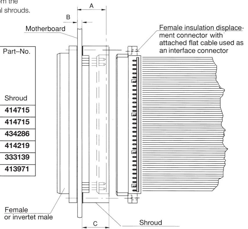
The female insulation displacement connector can be screwed to the shroud with a cheese-head tapping screw B2.2 x 9.5 DIN 7971.
