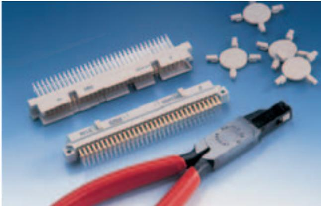
The coding tabs are inserted into existing slots on the female connector. By using coding pliers, the corresponding pre-notched area on the male connector is recessed.
