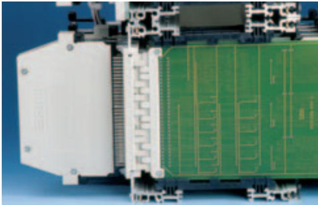
Coding Strip F mounted in a 19" sub-rack.
