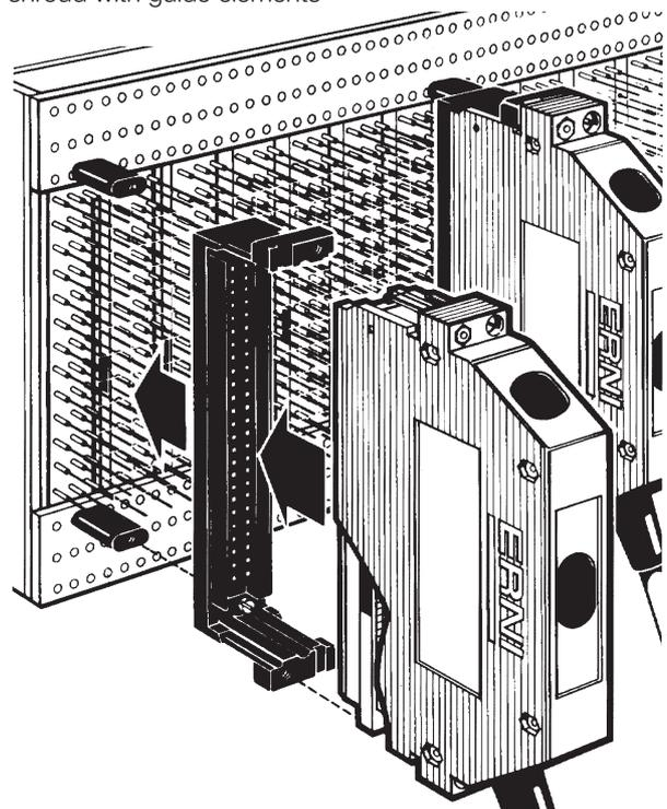
The female connector housings of size C, C/2 and E 160 fit into the cable connector housings of series KSG 173 and KSG 193.
