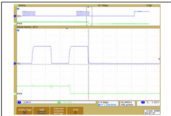
FIGURE 2-46: 100 k \Omega – Low-Voltage Decrement Wiper Settling Time ( V_{DD} = 2.7\text{V} ) ( 1\ \mu\text{s}/\text{Div} ).
