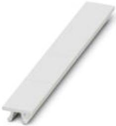
Zack marker strip, Strip, white, unlabeled, can be labeled with: Plotter, Mounting type: Snap into tall marker groove, for terminal block width: 22 mm, Lettering field: 10.5 x 21.8 mm
