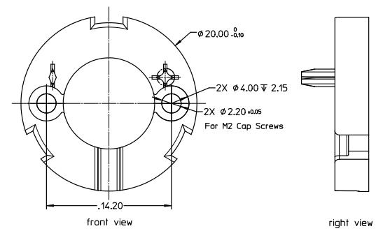
**CAUTION:** For optimal performance, base plate and plastic housing assembly are designed for a ONE time assembly process only. Removal and re-assembly process should be avoided due to the potential weakness of the latch after re-assembly.
