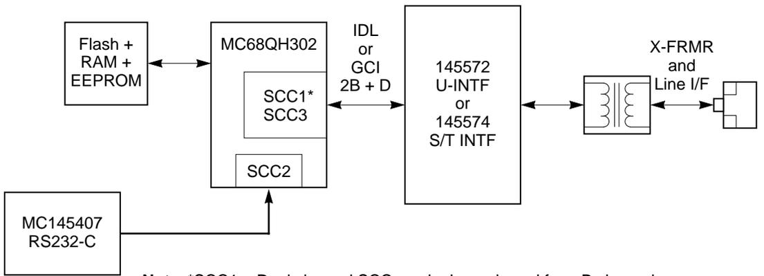
**Note:** \*SCC1 = Dual channel SCC, each channel used for a B channel
