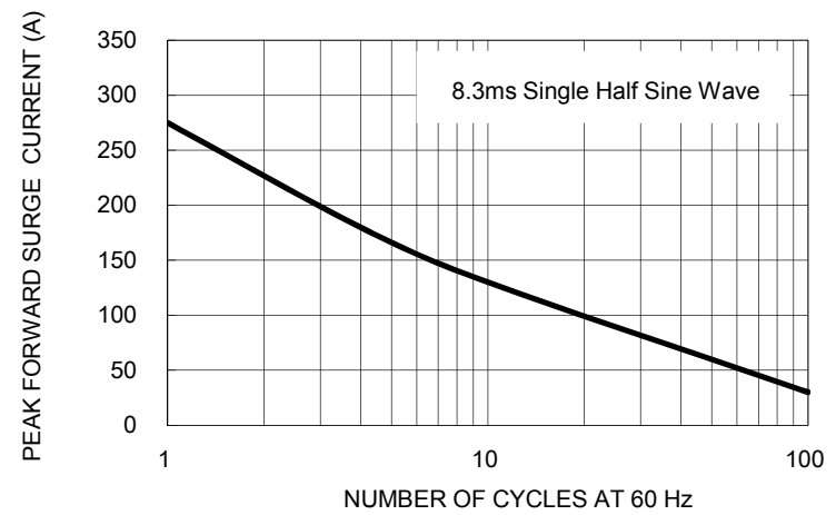
FIG. 2 MAXIMUM NON-REPETITIVE FORWARD SURGE CURRENT
