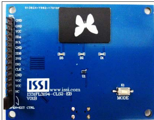
Figure 1: Photo of IS31FL3194 Evaluation Board
