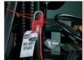
Immobilize large or cumbersome devices, such as forklifts
