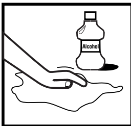
1) Clean surface with a clean cloth and isopropyl alcohol.
