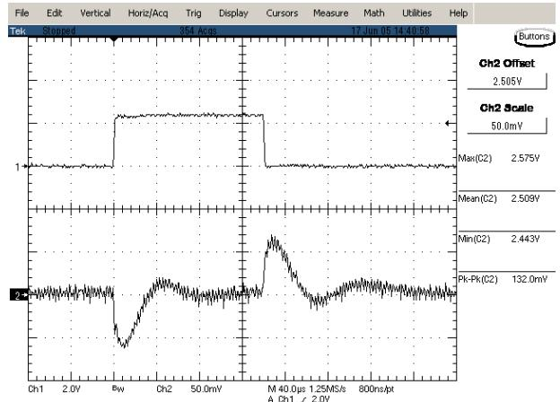
**Figure 22:** Typical transient response to step load change at 10A/μS from 50% to 75% and 75% to 50% of  $I_o$ , max at 12Vin, 2.5V out
