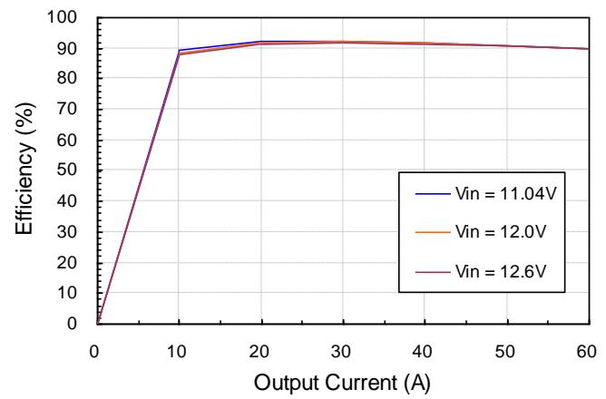
**Figure 4:** Converter efficiency vs. output current
