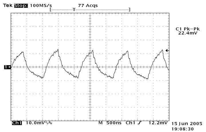
**Figure 10:** Output ripple & noise at 12Vin, 1.5V/60A out
