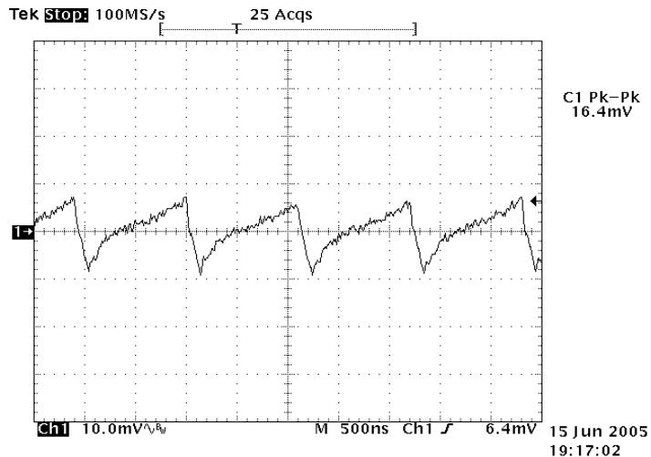
**Figure 13:** Output ripple & noise at 12Vin, 3.3V/60A out
