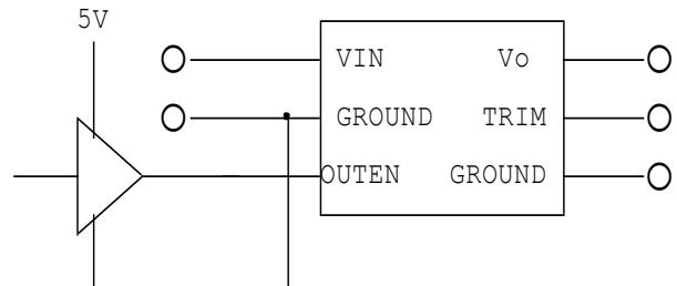
Figure 27: Remote ON/OFF Input Drive Circuit for Logic Driver
