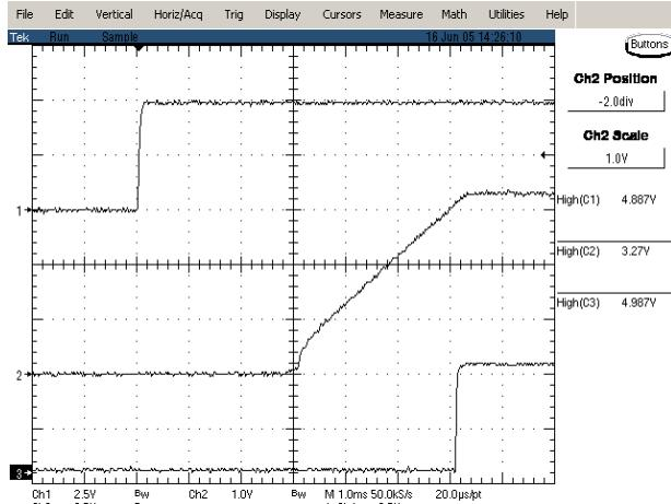
**Figure 17:** Turn on delay time at 12Vin, 3.3V/60A out
