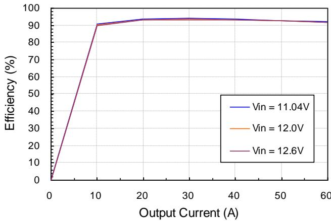
**Figure 5:** Converter efficiency vs. output current
