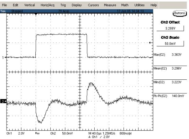
**Figure 23:** Typical transient response to step load change at 10A/μS from 50% to 75% and 75% to 50% of  $I_o$ , max at 12Vin, 3.3V out
