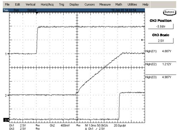
**Figure 16:** Turn on delay time Remote On/Off, 1.2V/60A out
