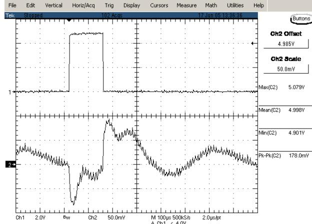
**Figure 24:** Typical transient response to step load change at 10A/μS from 50% to 75% and 75% to 50% of  $I_o$ , max at 12Vin, 5.0V out
