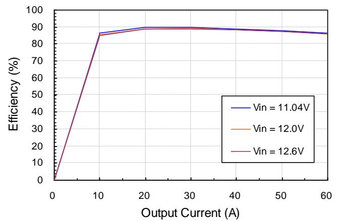
**Figure 2:** Converter efficiency vs. output current
