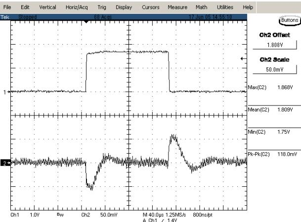
**Figure 21:** Typical transient response to step load change at 10A/μS from 50% to 75% and 75% to 50% of  $I_o$ , max at 12Vin, 1.8V out
