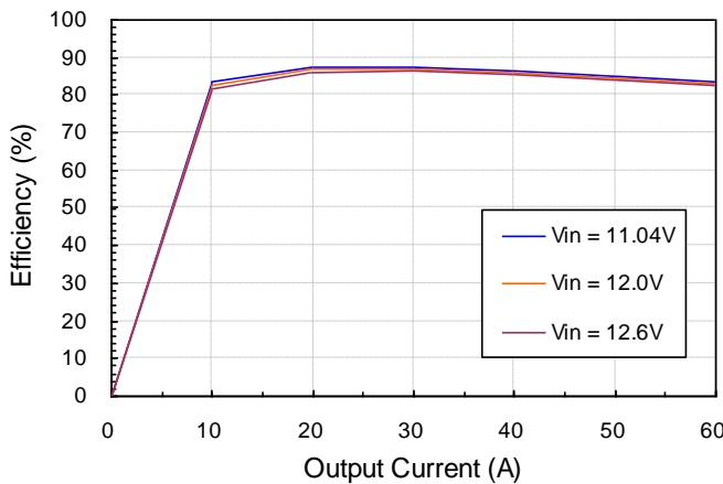
**Figure 1:** Converter efficiency vs. output current
