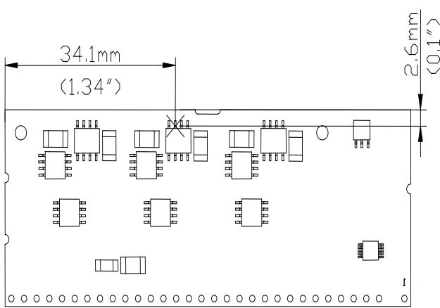
**Figure 36:** Temperature measurement location
