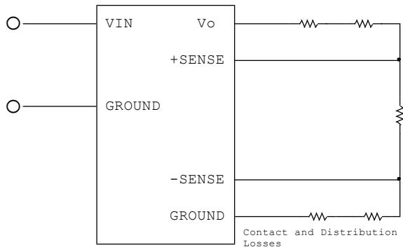
**Figure 29:** Effective circuit configuration for remote sense operation
