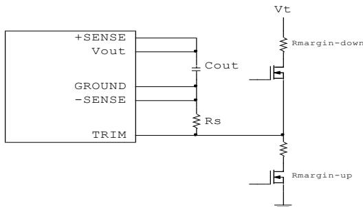
**Figure 34:** Circuit configuration for output voltage margining
