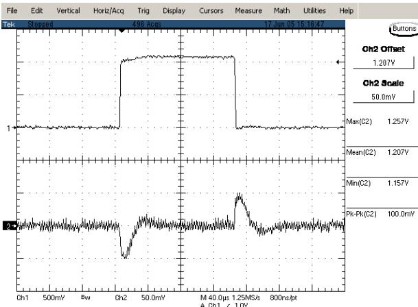
**Figure 19:** Typical transient response to step load change at 10A/μS from 50% to 75% and 75% to 50% of  $I_o$ , max at 12Vin, 1.2V out
