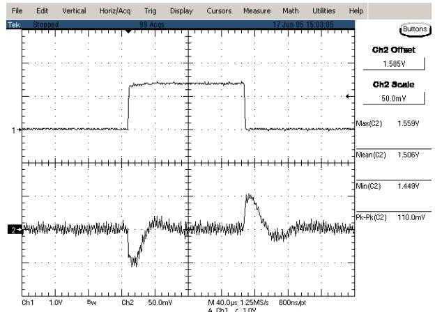
**Figure 20:** Typical transient response to step load change at 10A/μS from 50% to 75% and 75% to 50% of  $I_o$ , max at 12Vin, 1.5V out
