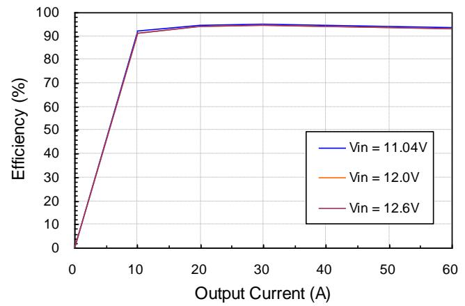
**Figure 6:** Converter efficiency vs. output current
