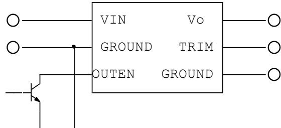
Figure 26: Remote ON/OFF Input Drive Circuit for Non-Isolated Bipolar
