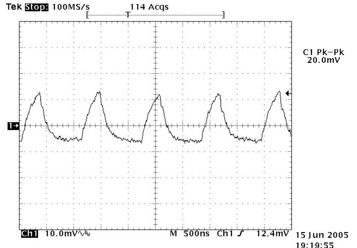
**Figure 14:** Output ripple & noise at 12Vin, 5V/60A out
