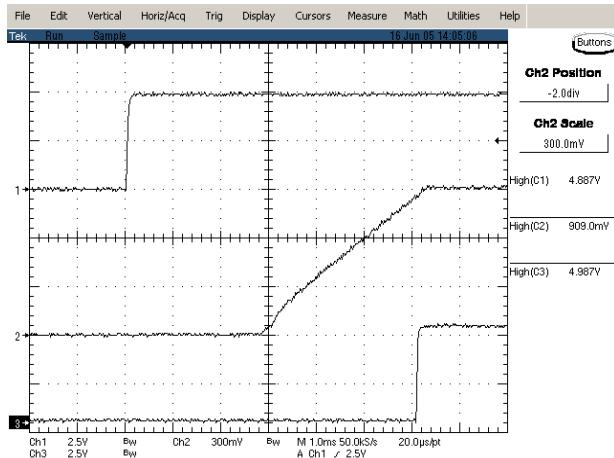
**Figure 15:** Turn on delay time at 12Vin, 0.9V/60A out
