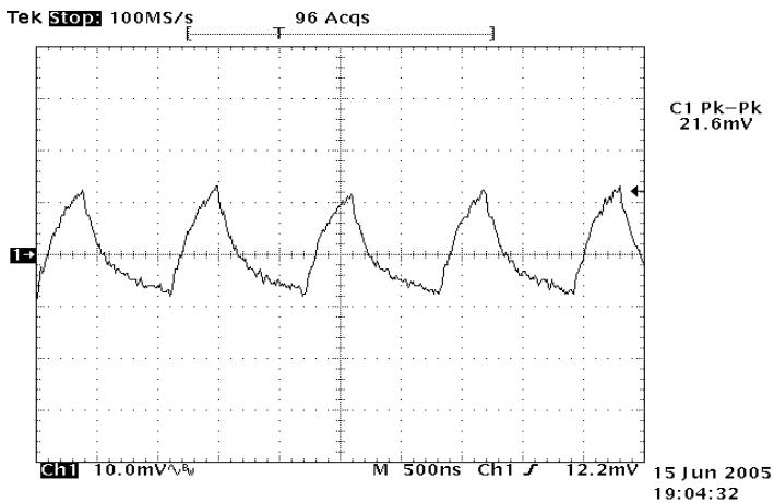
**Figure 9:** Output ripple & noise at 12Vin, 1.2V/60A out
