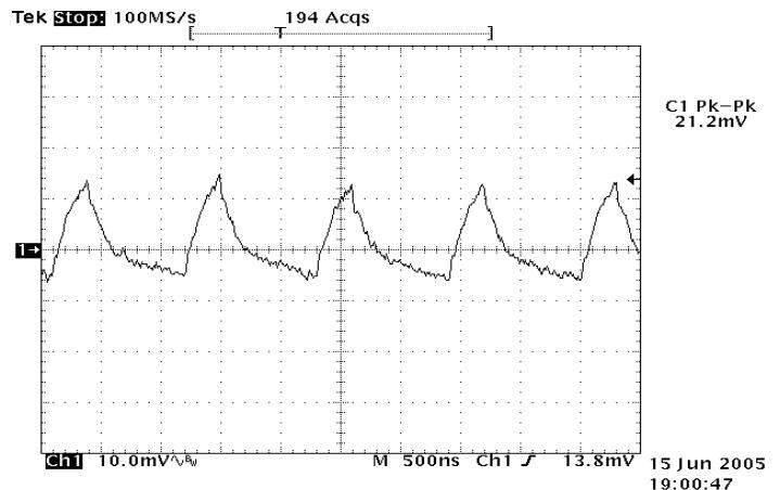
**Figure 8:** Output ripple & noise at 12Vin, 0.9V/60A out
