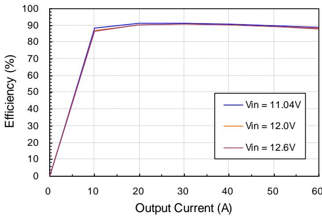
**Figure 3:** Converter efficiency vs. output current
