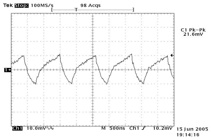
**Figure 12:** Output ripple & noise at 12Vin, 2.5V/60A out
