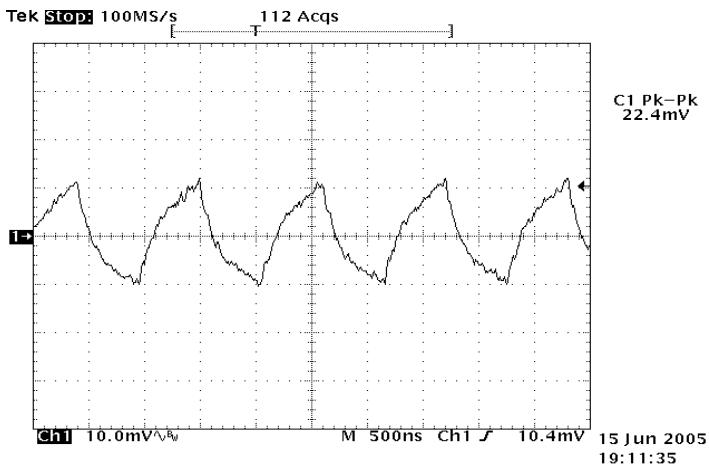
**Figure 11:** Output ripple & noise at 12Vin, 1.8V/60A out
