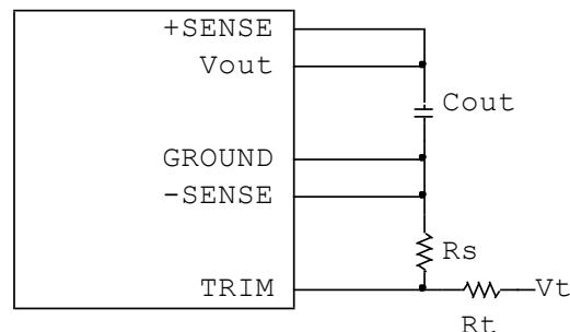
Figure 33: Trim Output Voltage – with Voltage Source
