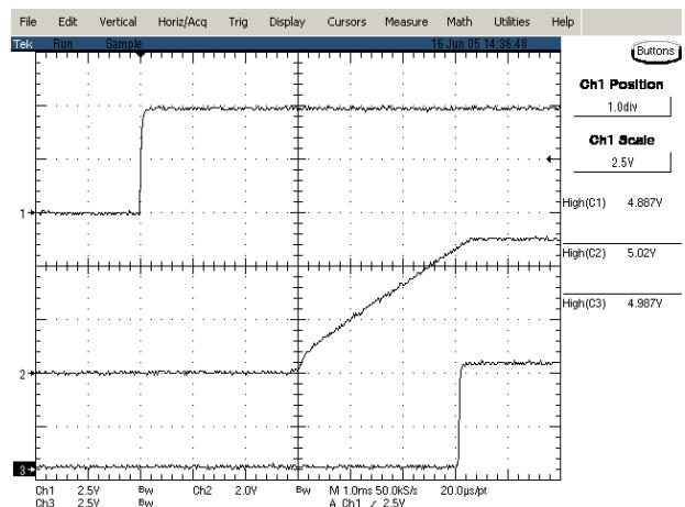
**Figure 18:** Turn on delay time Remote On/Off, 5V/60A out
