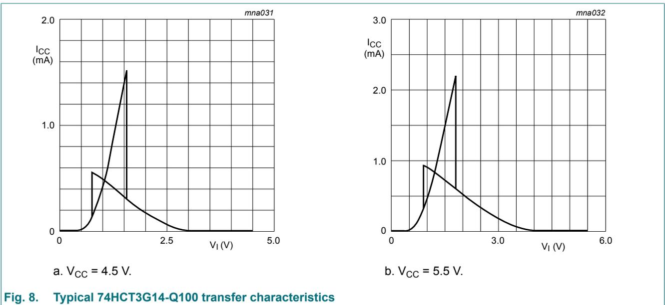
Fig. 8. Typical 74HCT3G14-Q100 transfer characteristics
