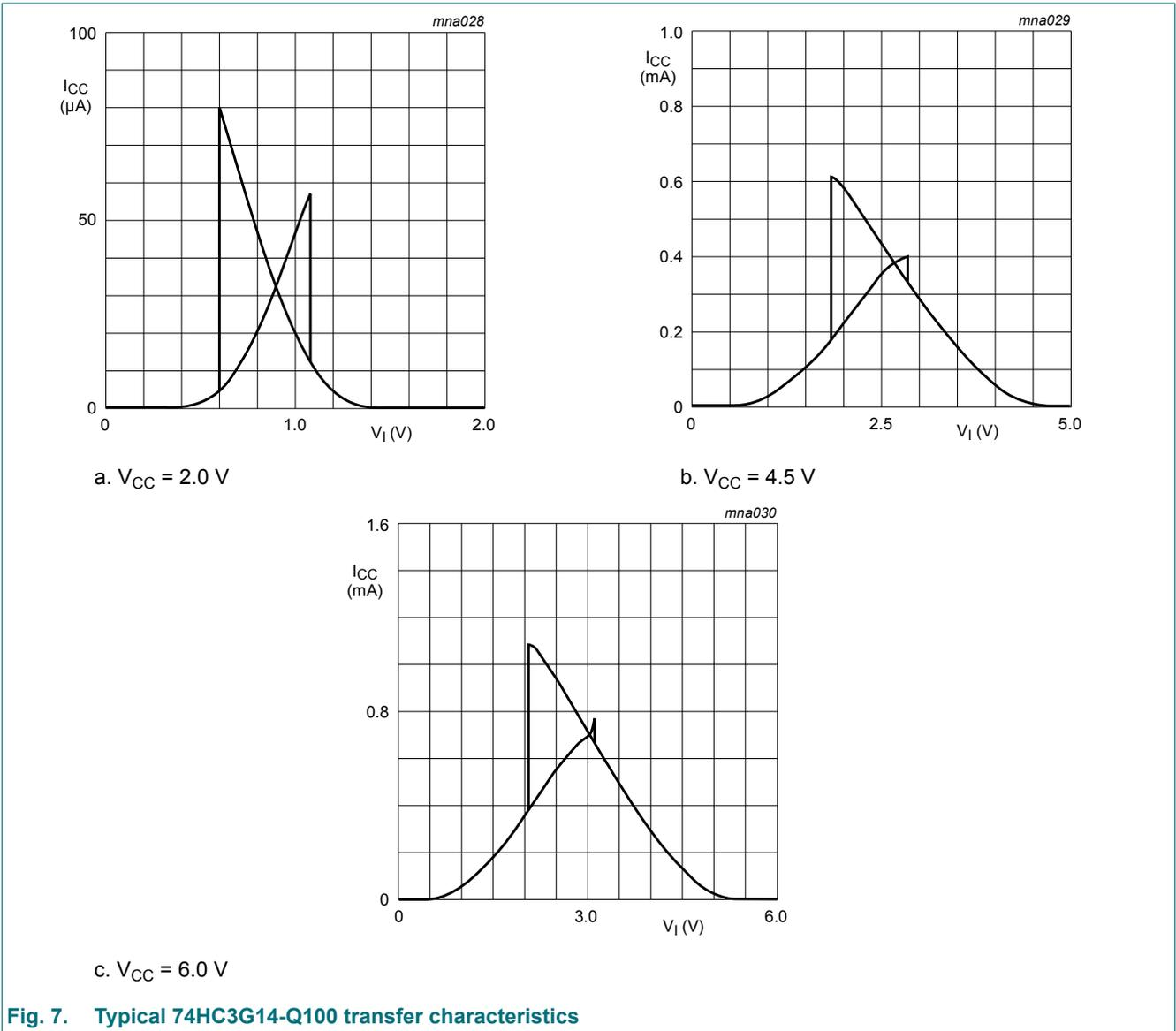
Fig. 7. Typical 74HC3G14-Q100 transfer characteristics
