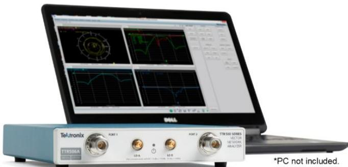
An independent RF source and three RF receivers for each port of the TTR500 enable you to take high-accuracy magnitude and phase measurements with a 1-port or 2-port device under test (DUT). Use the TTR500 to perform complete  $S_{11}$ ,  $S_{12}$ ,  $S_{21}$ , and  $S_{22}$  measurements of the DUT and display data in a variety of formats (see measurement functionality table).
