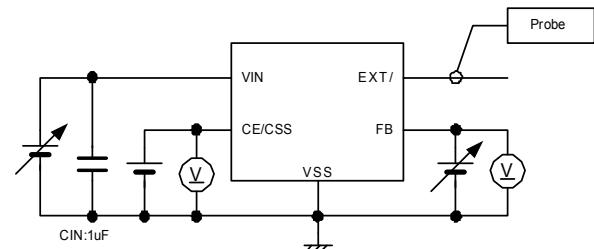
Circuit 3: Oscillation Frequency, PFMDUTY, U.V.L.O., Efficiency
