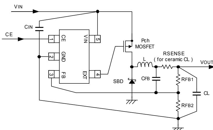
\* RSENSE : Tantalum and electrolytic capacitors can be used, in which case, RSENSE becomes unnecessary.
