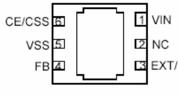
\* The dissipation pad for the USP-6C package (preliminary) should be solder-plated in recommended mount pattern and metal masking so as to enhance mounting strength and heat release. If the pad needs to be connected to other pins, it should be connected to the Vss (No.5) pin.
