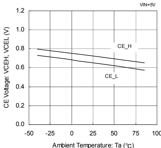
(16) CE Threshold vs. Input Voltage
