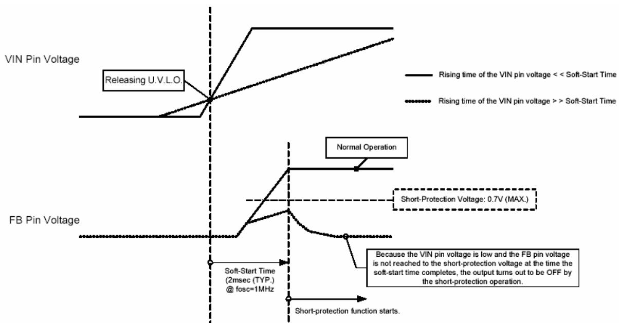
6. Use of the IC at voltages below the recommended minimum operating voltage may lead to instability.
