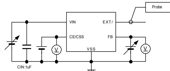
Circuit 3: Oscillation Frequency, PFMDUTY, U.V.L.O., Efficiency
