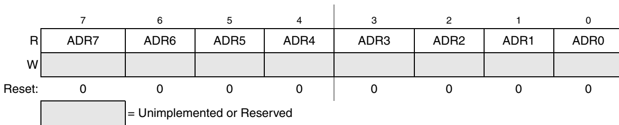
Figure 9-7. Data Result Low Register (ADCRL)
