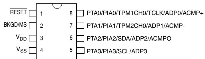
Figure 2-3. 8-Pin SOIC
