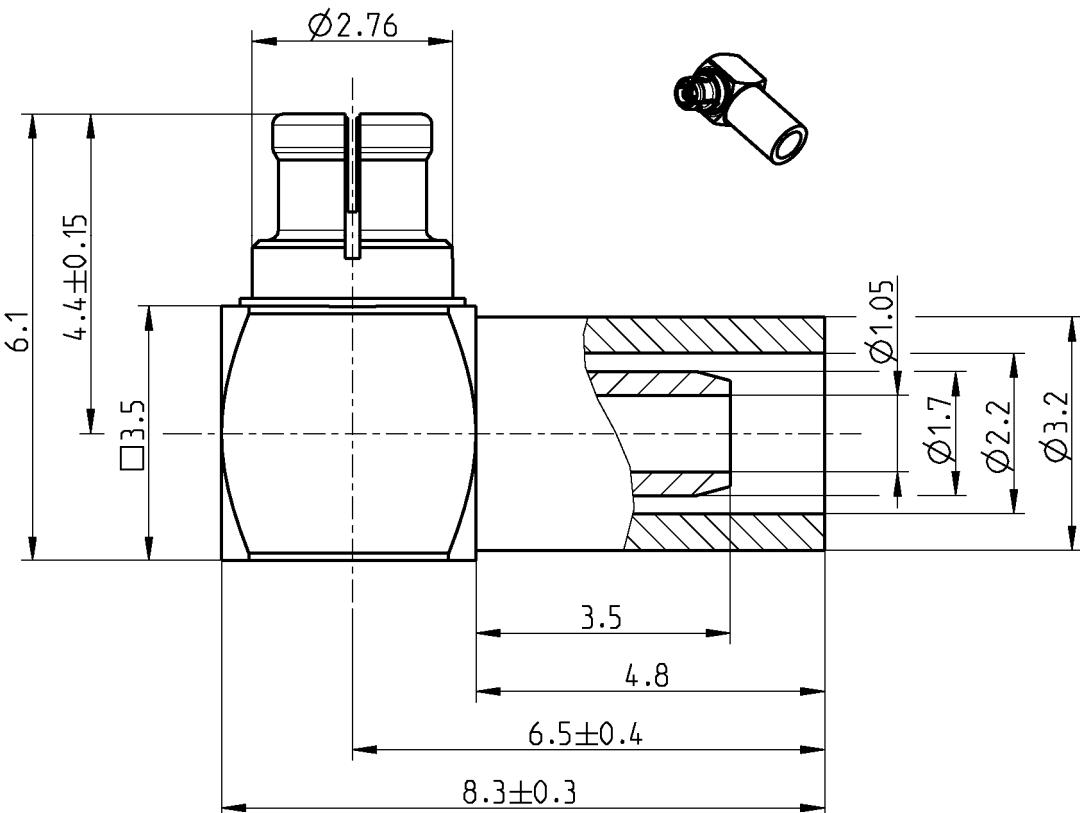
All dimensions are in mm; tolerances acc. ISO 2768 m-H
