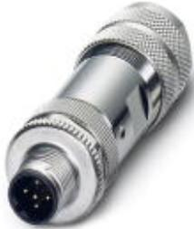
Bus system connector, male connector, straight, 5-pos., M12, shielded, gold-plated contacts, B-encoded, screw connection, metal knurl, PG11 cable gland
