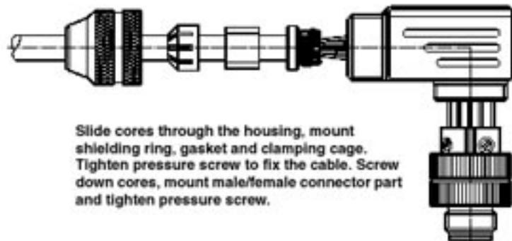
Slide cores through the housing, mount shielding ring, gasket and clamping cage. Tighten pressure screw to fix the cable. Screw down cores, mount male/female connector part and tighten pressure screw.
