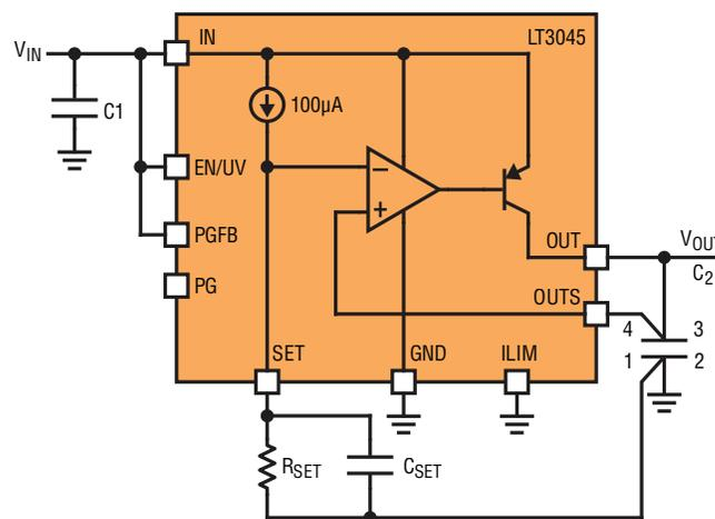
Figure 4. C2 and C<sub>SET</sub> Connections for Best Performance
