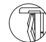
DETAIL VIEW VH1, VH3 & VH5 HOLE PLUGS (No wing serrations for ease of removal)
