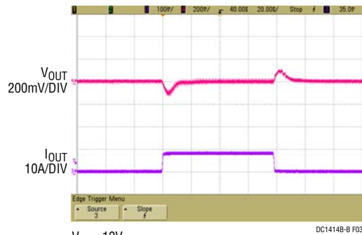
V_{IN} = 12V V_{OUT} = 1.2V 2A TO 10A LOAD STEP C_{OUT} = 2 \times 100\mu F, 3.6V, X5R, 1812 \text{ CERAMIC} + 1 \times 22\mu F, 10V, X5R, 1206 \text{ CERAMIC}
